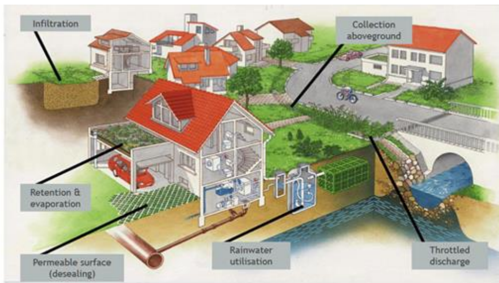
Figure 25: Example of on-site collection, retention and reuse of the young water infiltration of rainwater with decentralised rainwater management in urban areas ( Technical Training Manual on Urban Circular Water Management for Municipalities – Association for Rainwater Harvesting and Water Utilisation – INTERREG project – 2019 )
