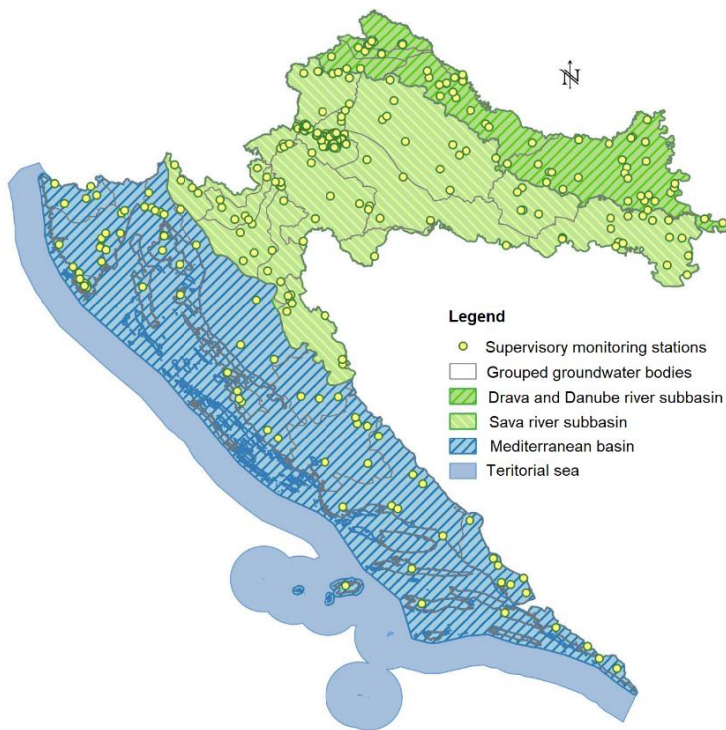
Fig. 10 Groundwater supervisory monitoring stations
