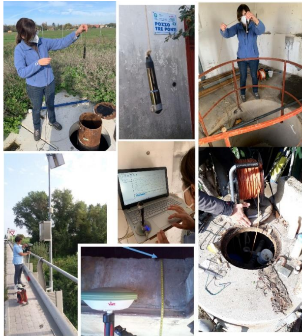
Fig. 2.5 Photos taken during the measurements of coordinates, elevation, water table level and vertical logs.
