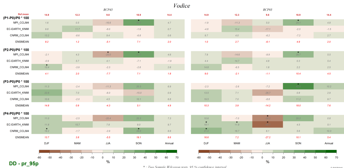
Figure 5-93: Seasonal and annual 95 th percentile of precipitation (intense precipitation) obtained by dynamical downscaling for Vodice: Ref. mean is 20 year simulated period (1986-2005) for ensemble mean in \text{mm day}^{-1} ; P1-P0, P2-P0, P3-P0, P4-P0 are changes (in %) in the future for following periods P1: 2021-2040, P2: 2041-2060, P3: 2061-2080, P4: 2081-2100. Differences are shown for individual models. Significant change is marked by star. Change is also shown as ensemble mean (ENSMEAN), not tested for significance. Left column is for RCP4.5 scenario and right for RCP8.5 scenario.
