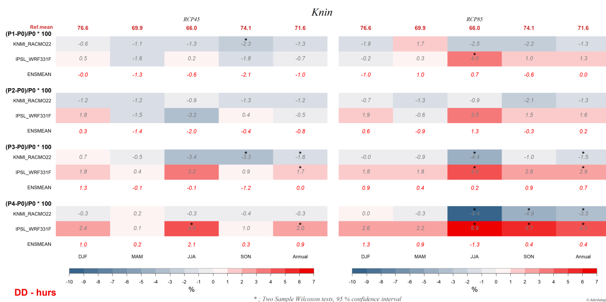
Figure 5-17: Seasonal and annual mean surface relative humidity (in %) obtained by dynamical downscaling for Knin: Ref. mean is 20 year simulated period (1986-2005); P1-P0, P2-P0, P3-P0, P4-P0 are relative changes in the future for following periods P1: 2021-2040, P2: 2041-2060, P3: 2061-2080, P4: 2081-2100. Differences are shown for individual models. Significant change is marked by star. Change is also shown as ensemble mean (ENSMEAN), not tested for significance. Left column is for RCP4.5 scenario and right for RCP8.5 scenario.
