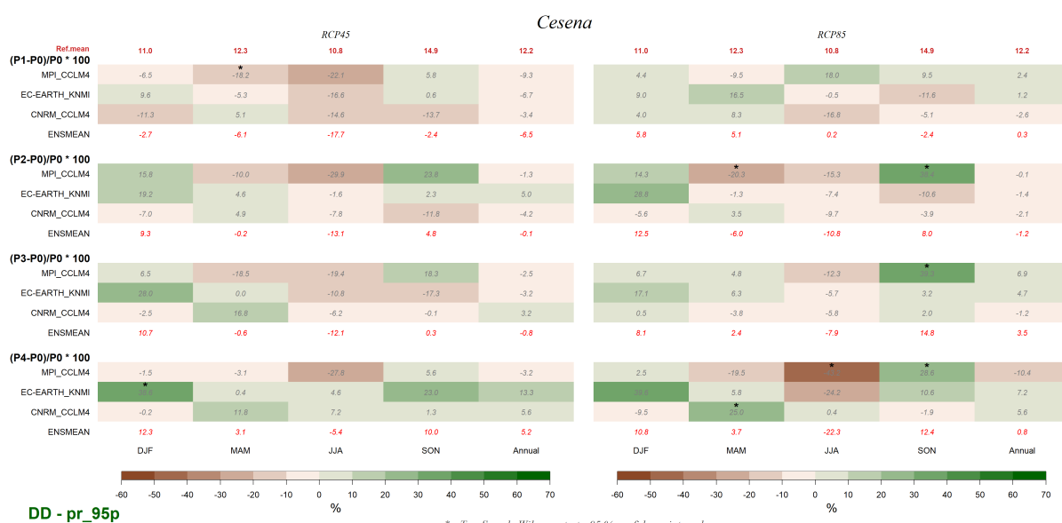
Figure 5-177: Seasonal and annual 95 th percentile of precipitation (intense precipitation) obtained by dynamical downscaling for Cesena: Ref. mean is 20 year simulated period (1986-2005) for ensemble mean in \text{mmday}^{-1} ; P1-P0, P2-P0, P3-P0, P4-P0 are changes (in %) in the future for following periods P1: 2021-2040, P2: 2041-2060, P3: 2061-2080, P4: 2081-2100. Differences are shown for individual models. Significant change is marked by star. Change is also shown as ensemble mean (ENSMEAN), not tested for significance. Left column is for RCP4.5 scenario and right for RCP8.5 scenario.
