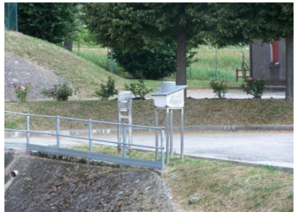
Figure 2.3-4 Detail of the historic station with totalizing rain gauge and recording rain gauge
