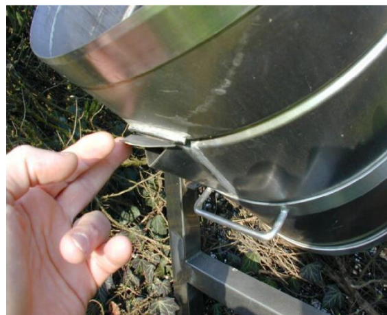
Figure 2.2-5 Totalizer rain gauge type C. 10: front view and detail of the opening spout for emptying the water into a graduated cylinder.
