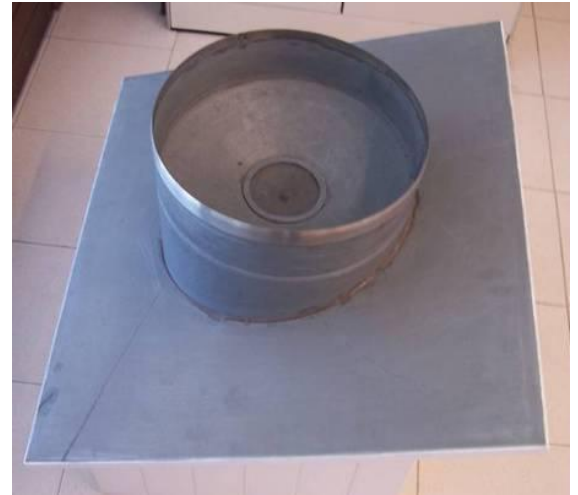
Figure 2.2-7 Detail of the precipitation capture funnel for M 20 type logger pluviograph located on the roof of the wooden shed. Capturing surface 1000 cm 2 diameter 35.7 cm
