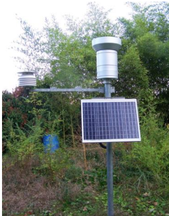
Figure 2.3-44 Strà thermo-pluviometric station seen from the North and South
