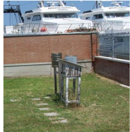
Figure 2.3-37 The historic station of Chioggia in 2020 at the time of replacement with the new instrumentation. Since 2004 the totalizing rain gauge and the pluviograph remained operational.
