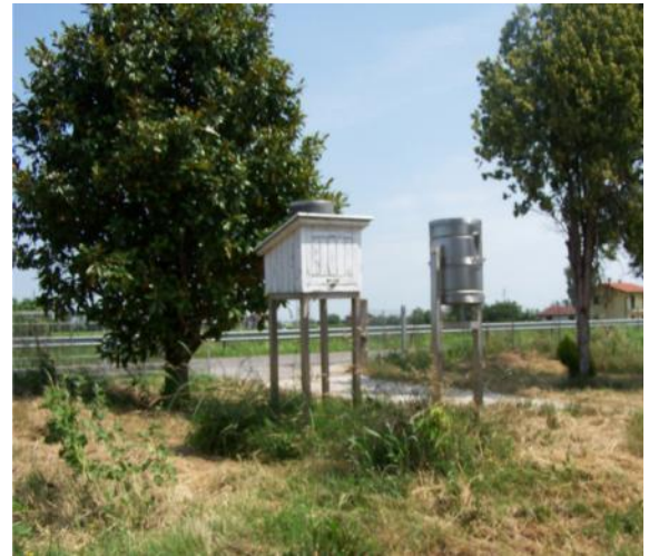
Figure 2.3-13 Detail of the historic station with recording rain gauge and totalizer rain gauge.
