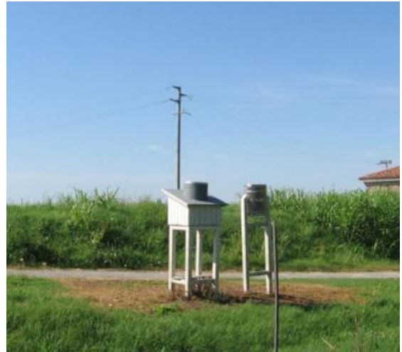
Figure 2.3-28 Detail of the historic station with recording rain gauge and totalizer rain gauge.
