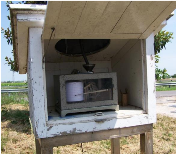
Figure 2.2-6 The pluviograph inside the wooden shed - Cortellazzo station year 2019.
