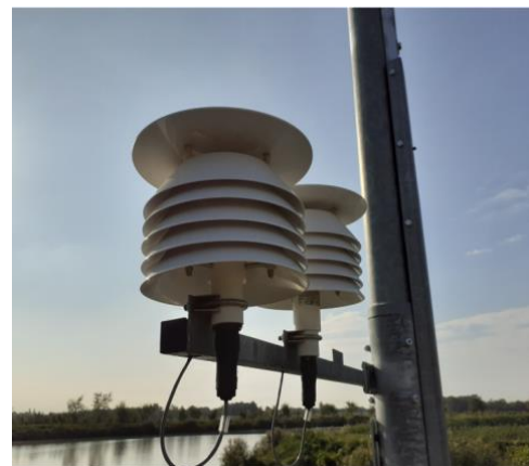
Figure 2.3-25 Detail of the screens of the Temperature and Relative Air Humidity sensors
