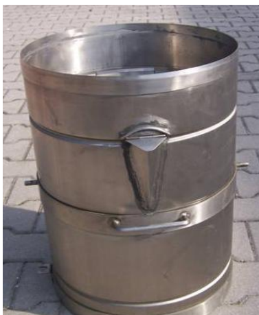
Figure 2.2-5 Totalizer rain gauge type C. 10: front view and detail of the opening spout for emptying the water into a graduated cylinder.
