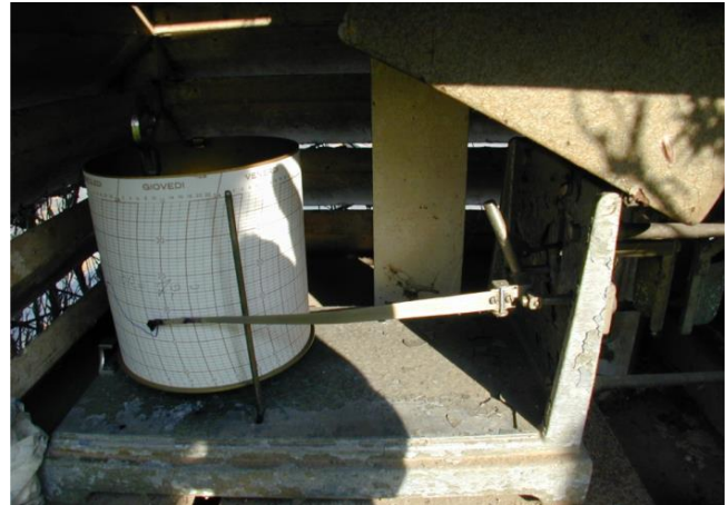
Figure 2.3-43 Strà thermometric station detail of the bimetallic foil thermograph operating in this station in 2003.
