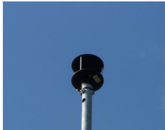
Figure 2.3-17 Detail of the sonic sensor measuring the direction and speed of the wind at 10 m above the ground
