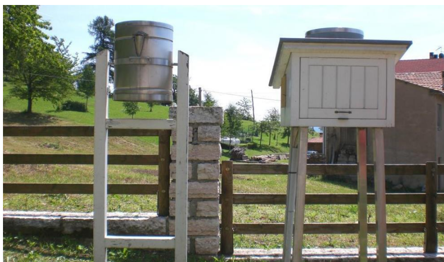
Figure 2.2-2 Historical rain gauge station; on the left totalizer rain gauge and on the right recording rain gauge both built by the Strà workshop.
