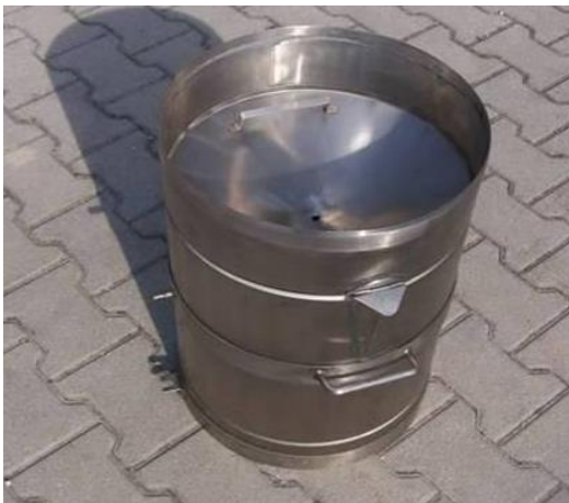
Figure 2.2-3 Totalizer rain gauge C. 10 with absorbing surface of 1000 cm 2 diameter 35.7 cm with conical lid inserted about 10 cm from the upper edge
