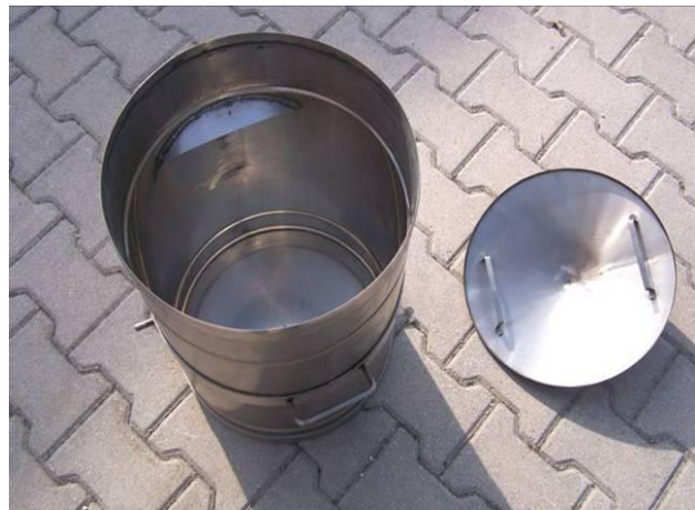
Figure 2.2-4 Totalizer rain gauge C. 10 with cover removed, in configuration for the measurement of snowfall.
