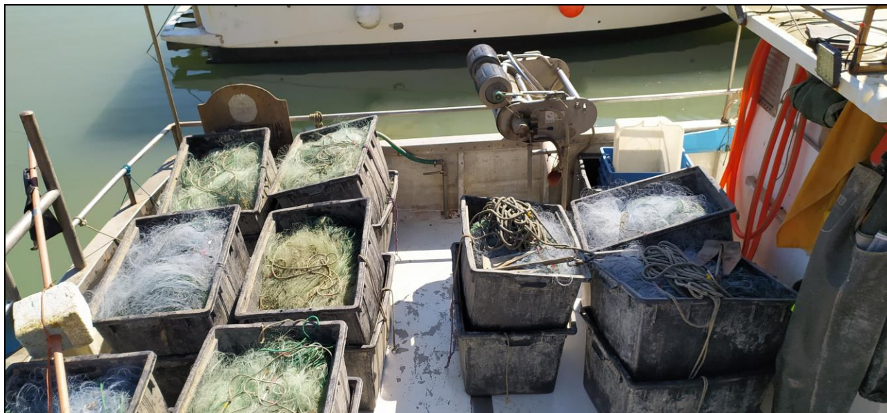
Figure 13 - Gill nets in the plastic boxes, ready to be deployed; the roller machine used for ordering the nets is also visible at center of the figure
