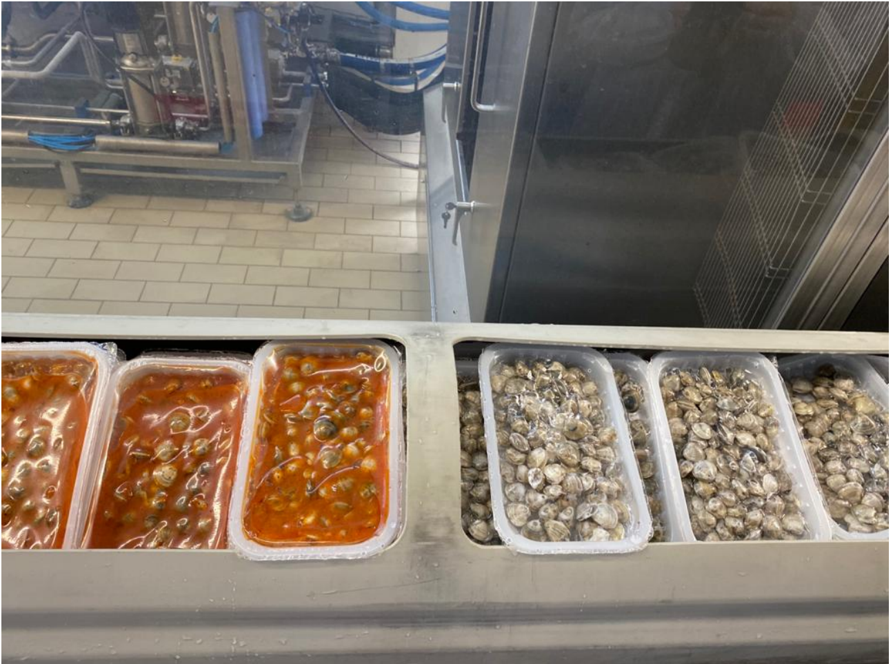
Figure 1. Samples of two different products based on the stuffed venus ( Chamelea gallina ) placed in the cylindrical tray prior the HPP treatment.
