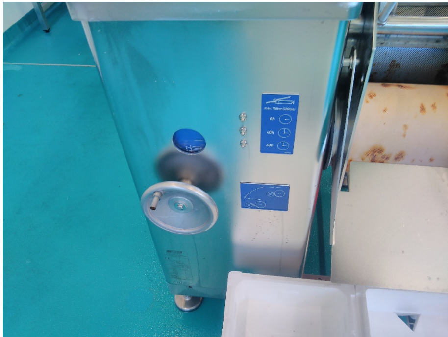
Figure 5. Pressure adjustment valve, Source: FC Istra photos
