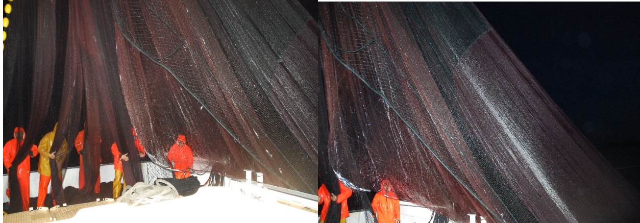
Pictures 86. and 87. Pulling the purse seine net out of the sea and stacking at the stern of the ship (photo Andrić V.)
