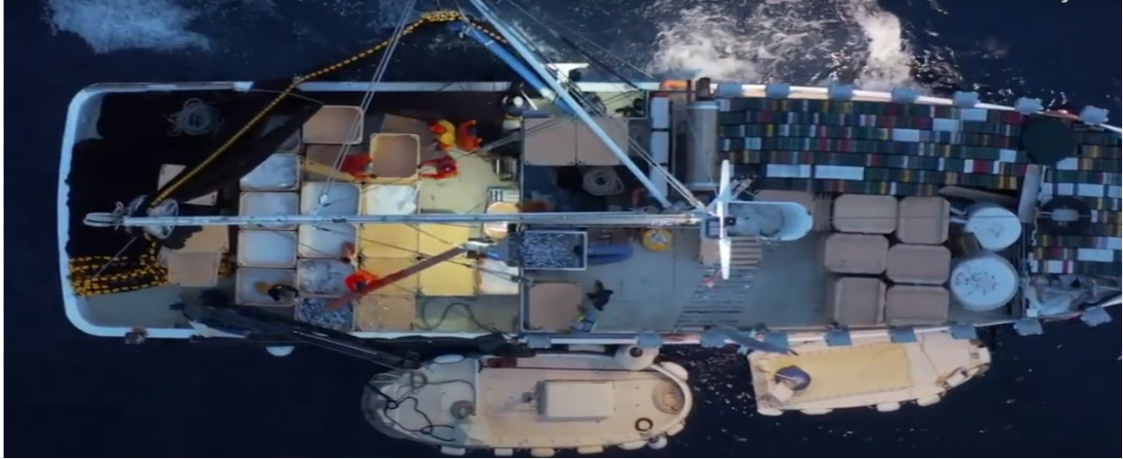
Picture 56. Filling thermal insulation bins with fish using a pump (photo Peraić L.)
