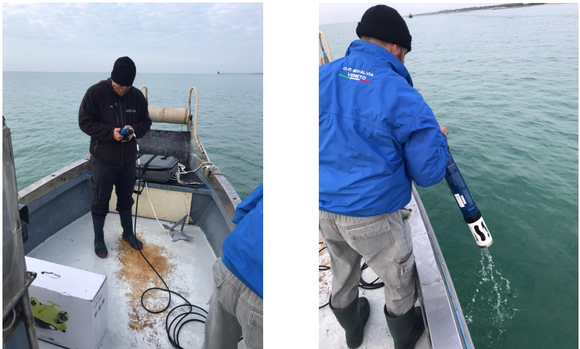
Figure: Measurement of water column properties with the multi-parameter probe.
