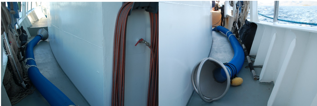
Pictures 44. and 45. Tube with funnel for catching fish (photo Lovrinov M.)
