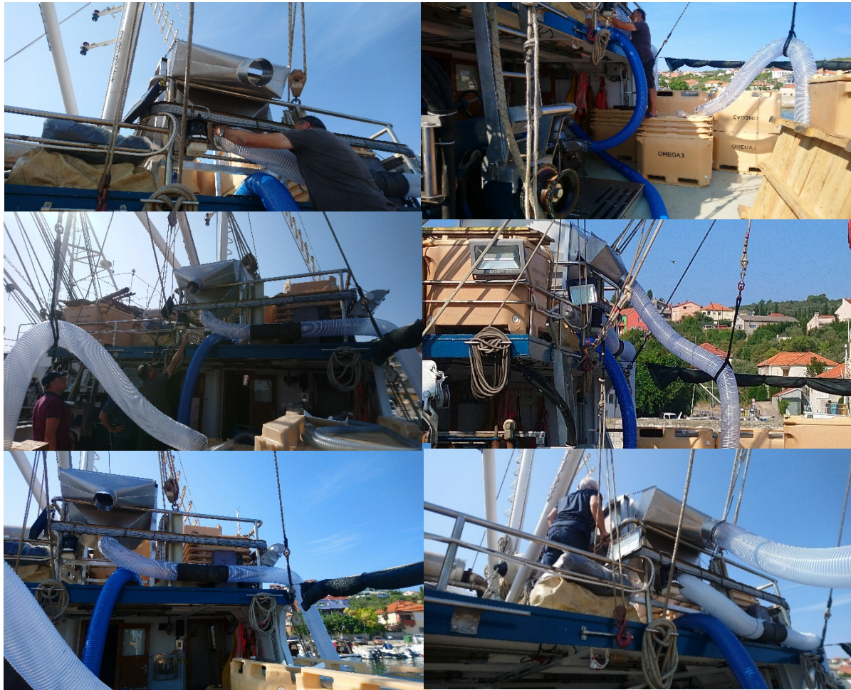
Pictures 38. ,39., 40. ,41., 42. and 43. Placement of the fish discharge unit on the cabin (photo Lovrinov M.)
