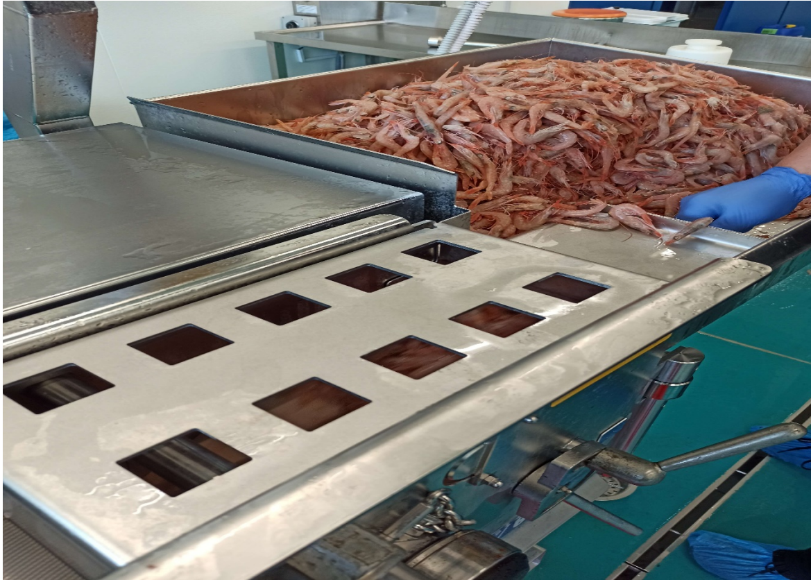
Figure 8. Separation of flesh – shrimp pulp and shell, Source: FC Istra photos
