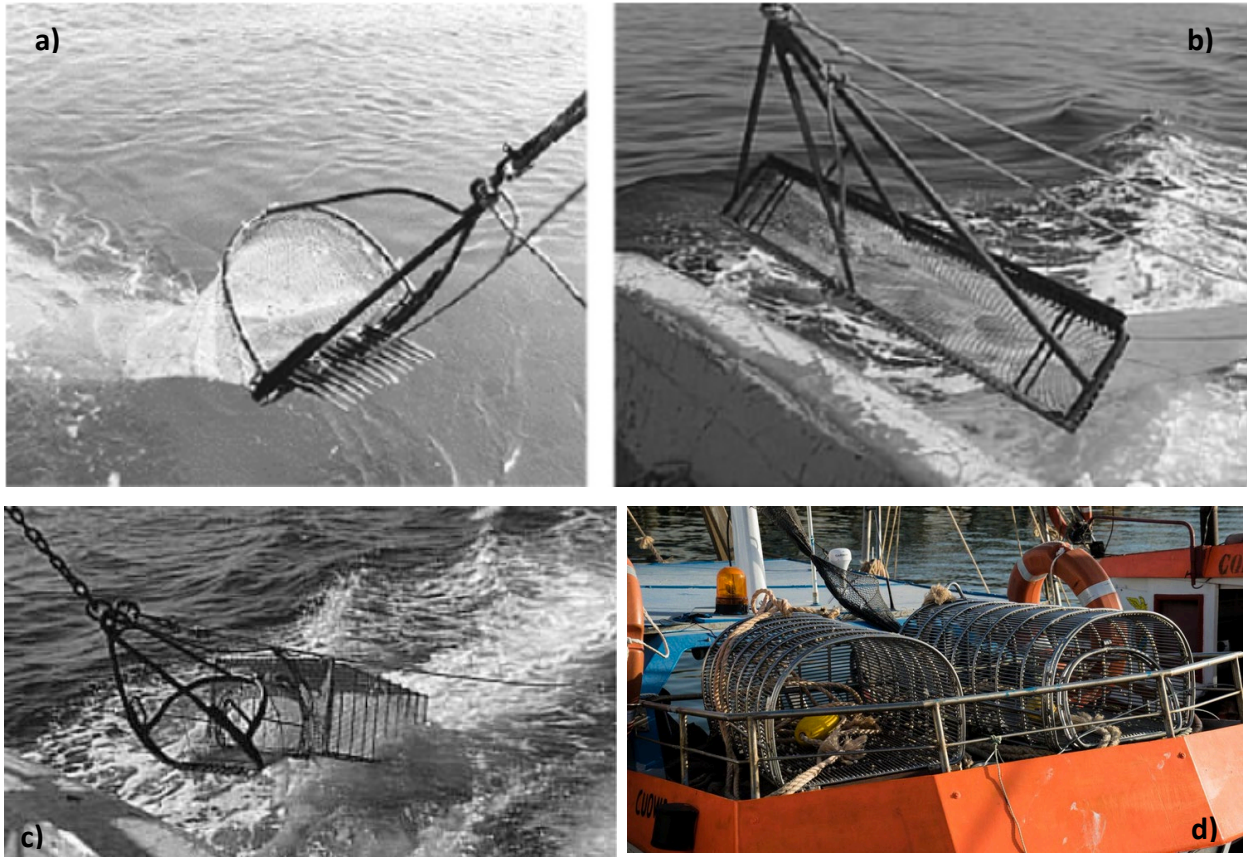
Figure 11. Examples of dredges used for clam fishery in Portugal: traditional dredge (a), dredge used in the north of Portugal (b), grid dredge, an improvement of the traditional dredge (c), modified fishing gear to reduce discards (d). Source: web
