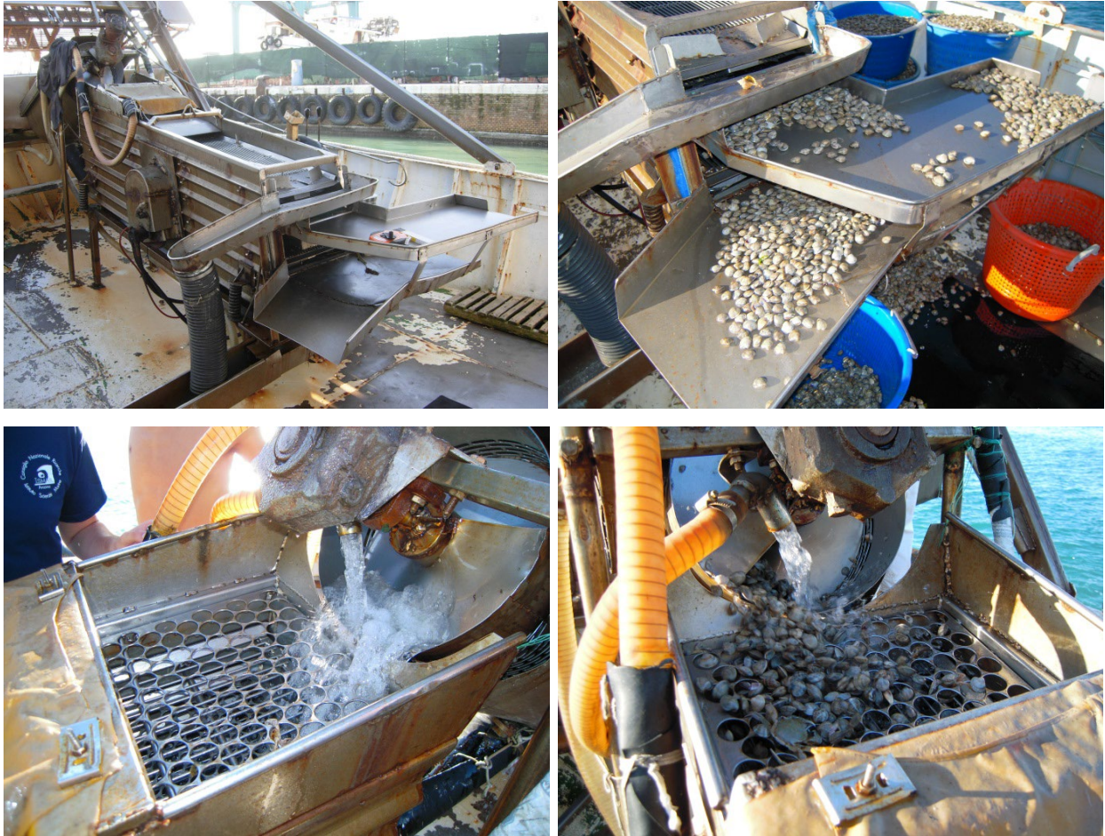
Figure 5,6,7,8 Details of the sorting multi-level sorting machine used on-board striped venus fishing vessels in Italy, Source: web
