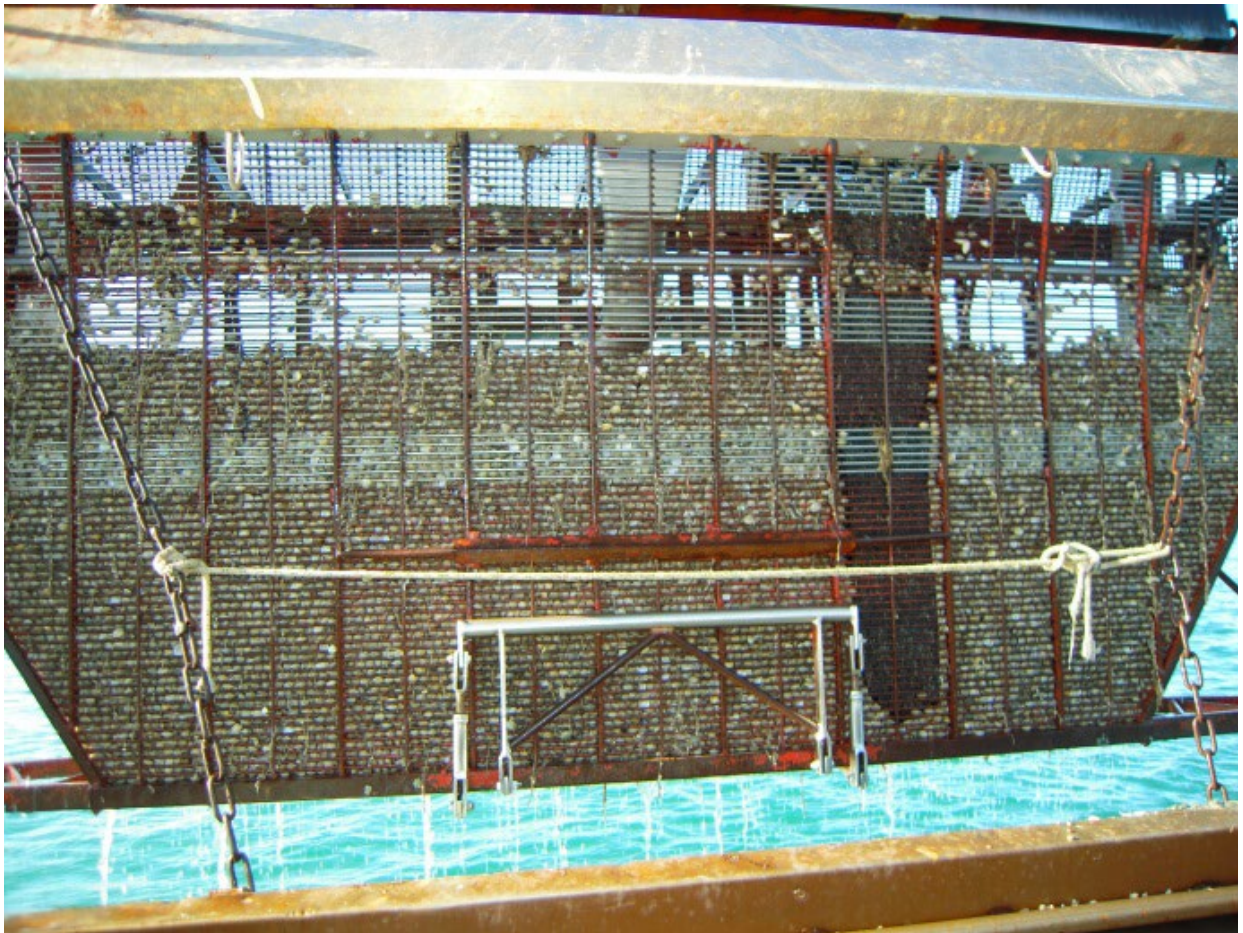
Figure 2. A detail of the construction of the hydraulic dredge cage and the sieving screens used.
