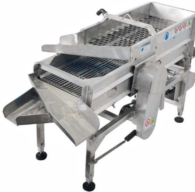
Figure 14. An example of a vibrating sorting machine used in Adriatic clam fishery, Source: web
