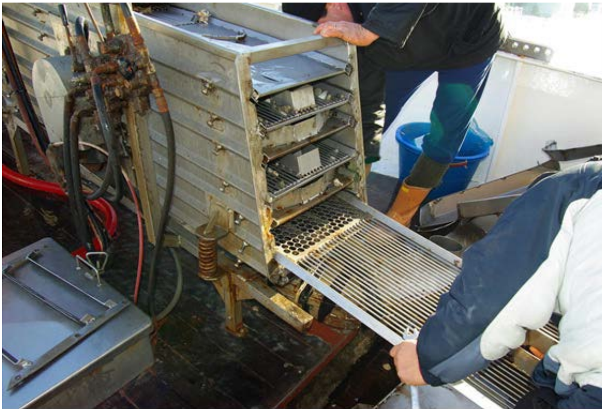
Figure 3. A multi-level vibrating sorting machine used on-board hydraulic dredge fishing vessels,
