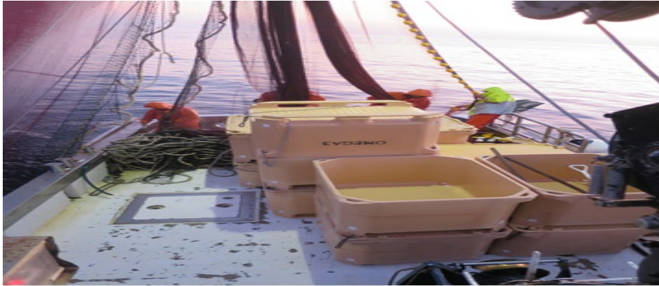
Figure 19. Deck of ship B with isothermal bins and opening of the tank for receiving fish below deck
