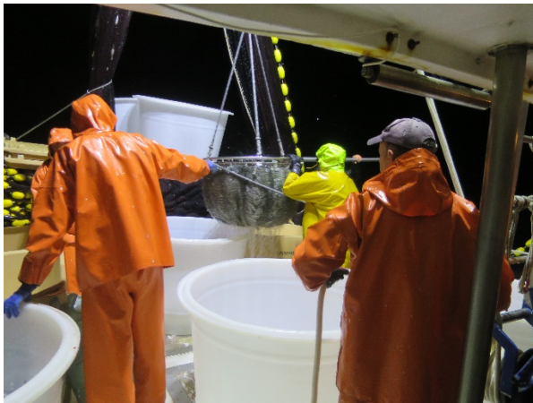
Figures 5,6,7 and 8. Transfer of fish by the traditional method using brailer - compacted fish flock in the net, filling the brailer, transfer of catch to the deck, release of catch into the cooling tank (photo Janči T.)
