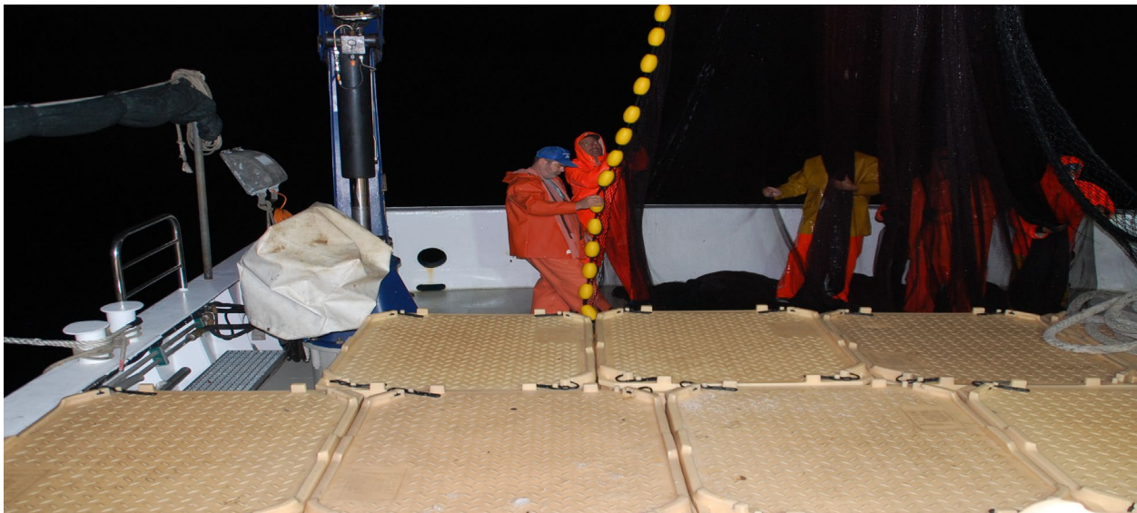
Figure 32. View of the arrangement of thermo bins and aft part for stacking the purse seine net (photo Andrić V.)
