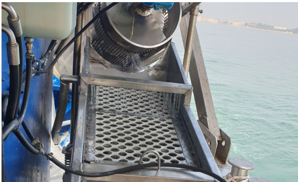
Figure 22. A preliminary implementation of sorting screens made of Teflon, Source: Web
