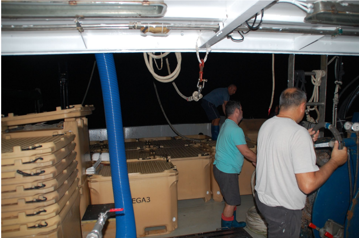
Figure 31. View of the arrangement of thermo insulation tanks and cramped space at the stern of the ship (photo Andrić V.)
