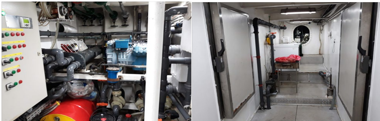
Figures 17 and 18. Ship's seawater cooling device and ship's ice and cold seawater tanks (source: WWF Adria)
