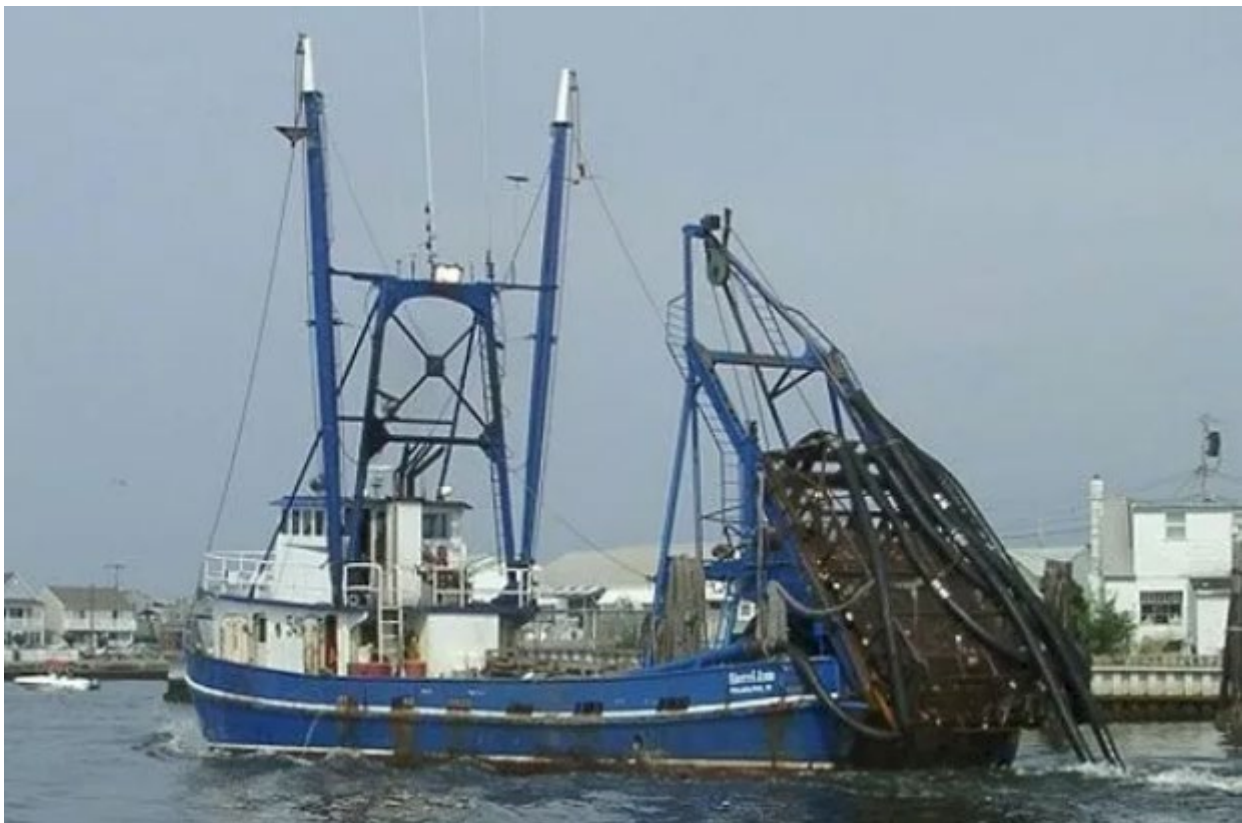
Figure 12. An example of a hydraulic dredge vessel in New England (USA) clam fishery. Source: web
