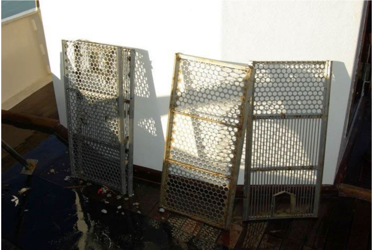
Figure 4. Examples of different interchangeable sorting screens, and combinations of different sorting meshes, Source: Web
