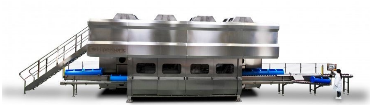
Figure 23. Hyperbaric chamber for high-pressure food processing (source: https://www.hiperbaric.com/en/hiperbaric420 )
