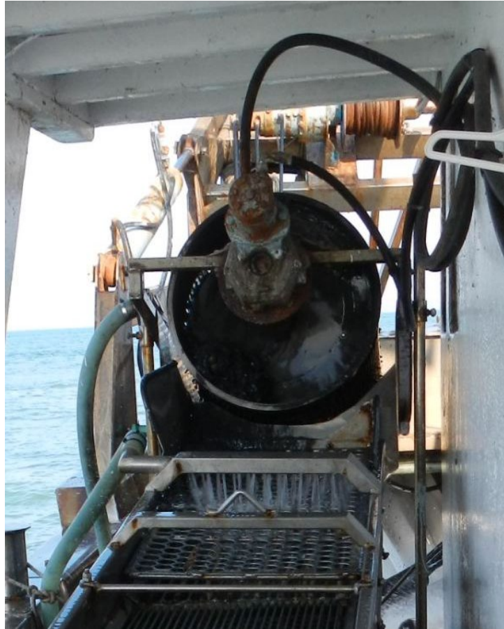
Figure 29. A view of the upward rotating sorting screw (above) and the vibrating sorting sieve (below) used for sorting the catch from the hydraulic dredge. [source: ISPRA, 2016]
