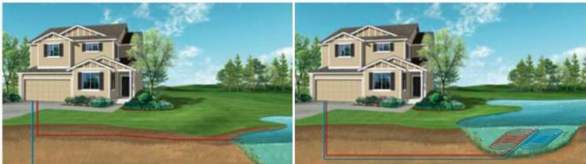
Figure 4-8 Open (left) and closed (right) version of the seawater heat pump system
