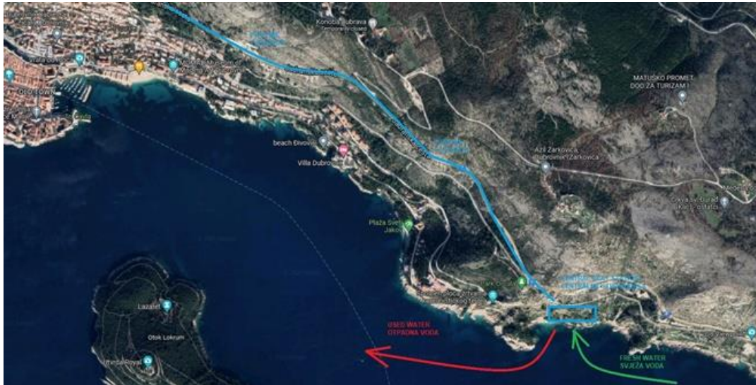
Figure 38: Preliminary concept of the heating and cooling pipe network of the pilot project
