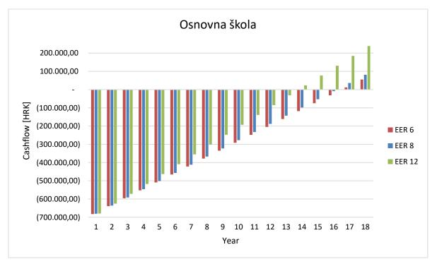
Figure 70 - Payback period for an elementary school in case of deployment of SWHP for heating and cooling
