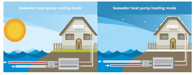
Figure 10 - Illustration of heating and cooling mode for seawater heat pumps [3]
