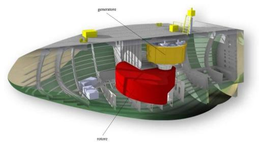
Figure 51 - Scheme of the Penguin device.
