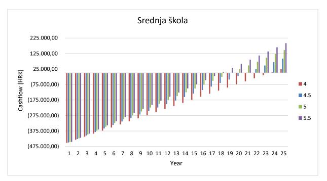
Figure 71 - Payback period for high school in case of deployment of SWHP only for heating
