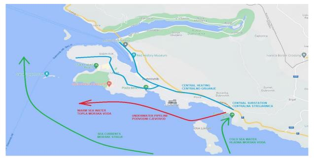
*Figure 73 - Heating pipelines in Dubrovnik*
