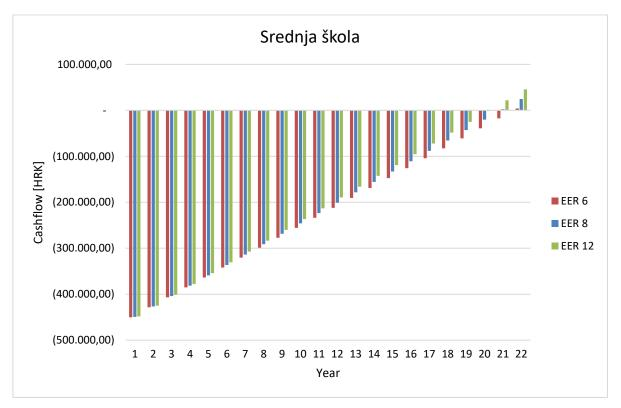
Figure 72 - Payback period for high school in case of deployment of SWHP for heating and cooling
