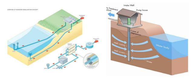
Figure 11 - Basic seawater heat pump system with direct water intake (left) and with the dwelling (right) [5]
