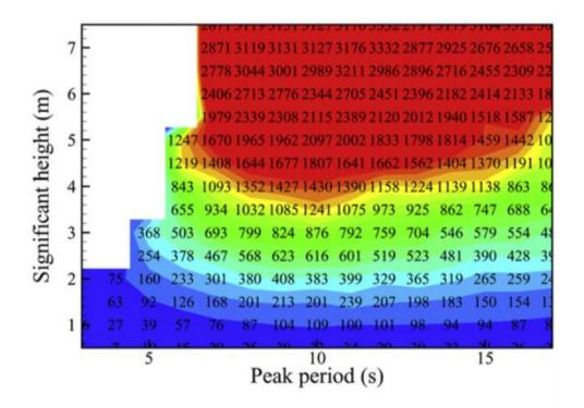
Figure 81 - Waveroller Power Matrix.
