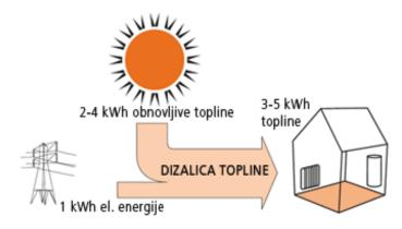
Figure 27 - Heat pump combined with solar panels that produce renewable energy
