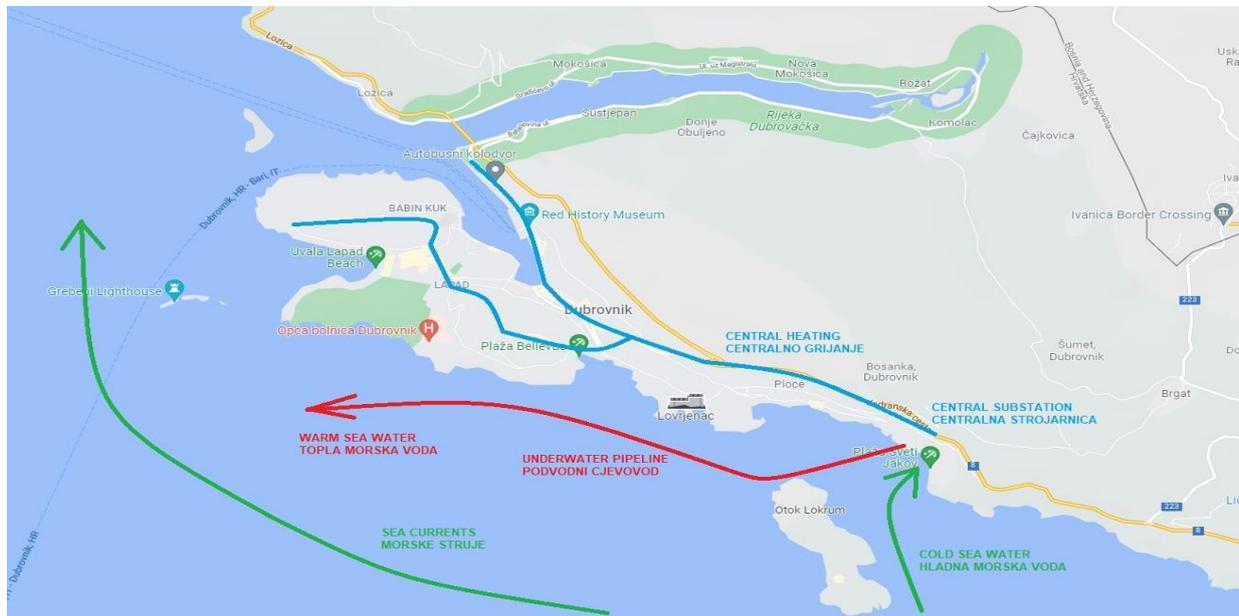
Figure 73 - Heating pipelines in Dubrovnik
