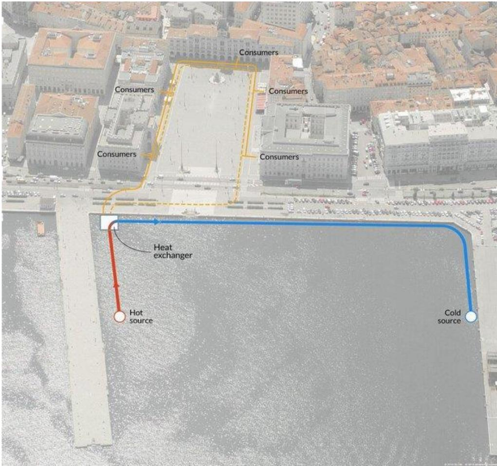
Figure 12 - Open-loop system for seawater heat pumps with the additional closed-loop distribution system [7]
