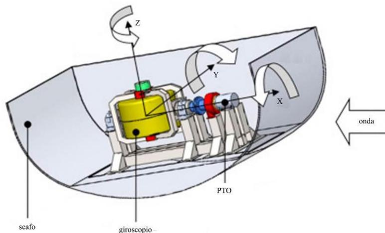
Figure 48 - Scheme of the ISWEC device.
