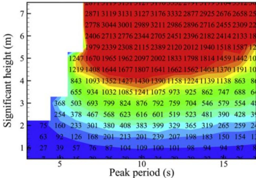
Figure 81 - Waveroller Power Matrix.
