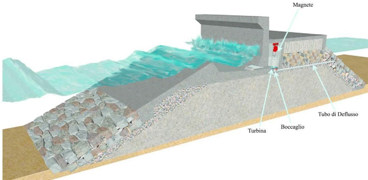
Figure 54 - Scheme of the OBREC system.
