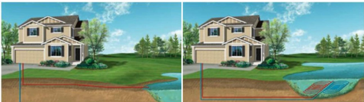
Figure 127 - Open (left) and closed (right) version of the seawater heat pump system
