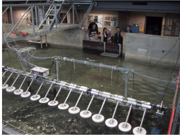
Figure 6 - Early scale 1:40 Wave Star Energy test model in the wave test tank at Aalborg University in 2004
