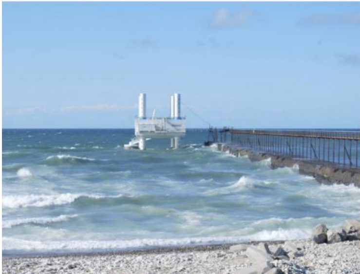
Figure 8 - The Wavestar prototype (above, a 2-float section of the full 20-float machine (below):
