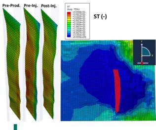
Fig 3. Fault Stability study outcome: Slip Tendency (left), Fault map (right)
