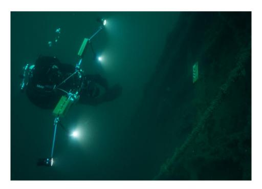
Photogrammetry is an optical based technology for estimating the 3D structure of a scene from 2D overlapping images, acquired by a moving sensor.
