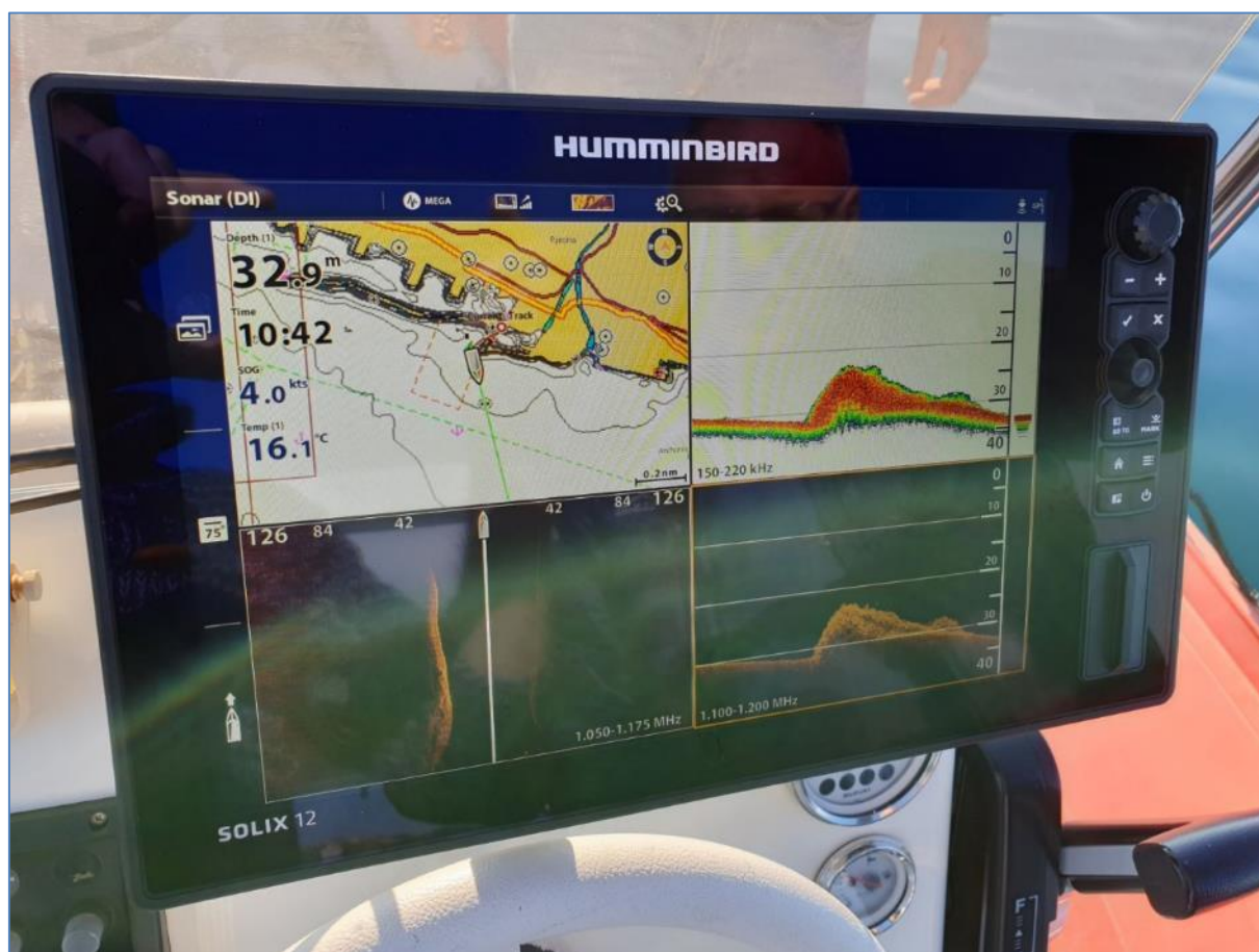
Figure 1. Side scan sonar Humminbird Solix
