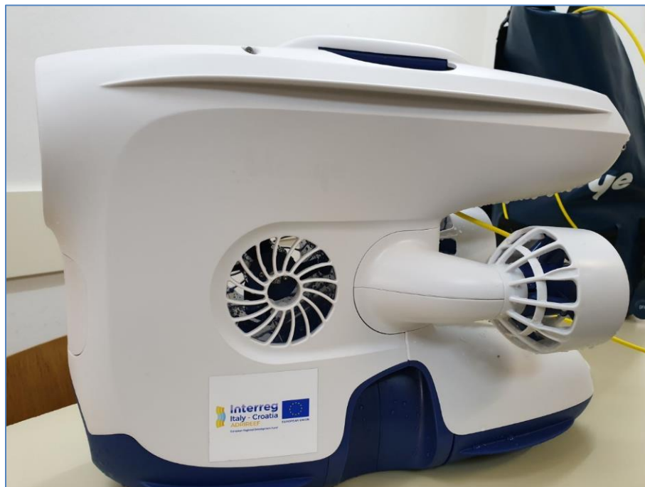
Figure 2. Underwater drone Blueye Pioneer
