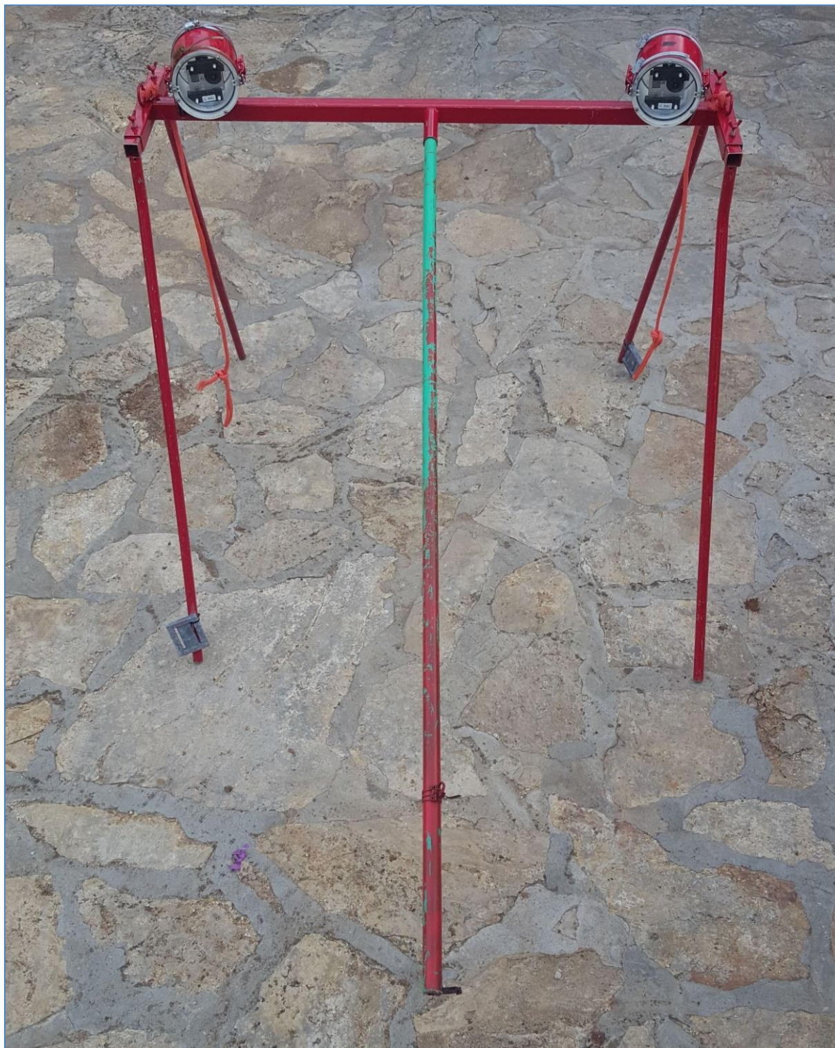
Figure 38 Stereo BRUV system used in research
