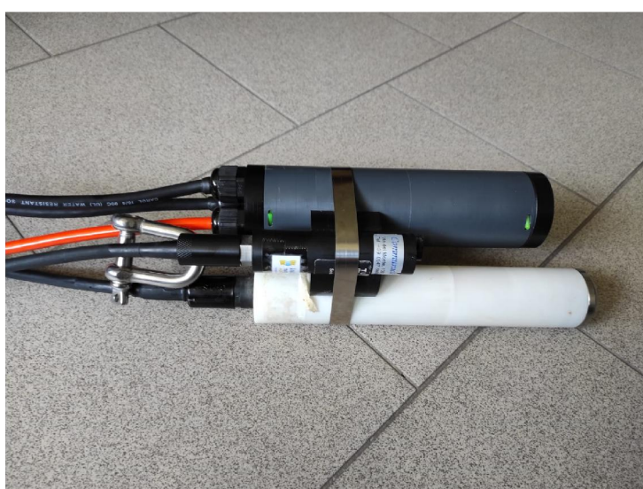
Figure 4 - Turner Turbidity probe mounted with other instruments.
