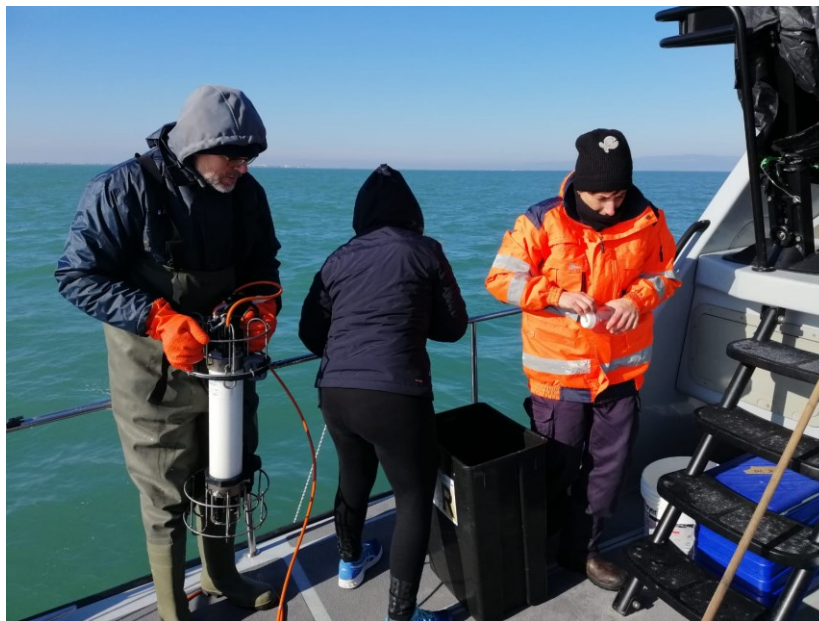
Fig. 12: Measurement of chemical-physical parameters by means of a multi-parameter probe and water sampling during autumn-winter time.
