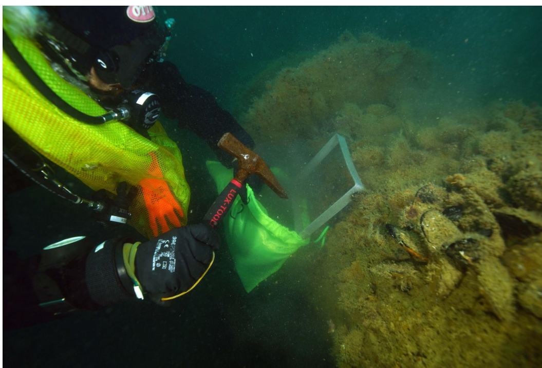
Figure 3.5 - Sampling benthic community by scraping standard surfaces.
