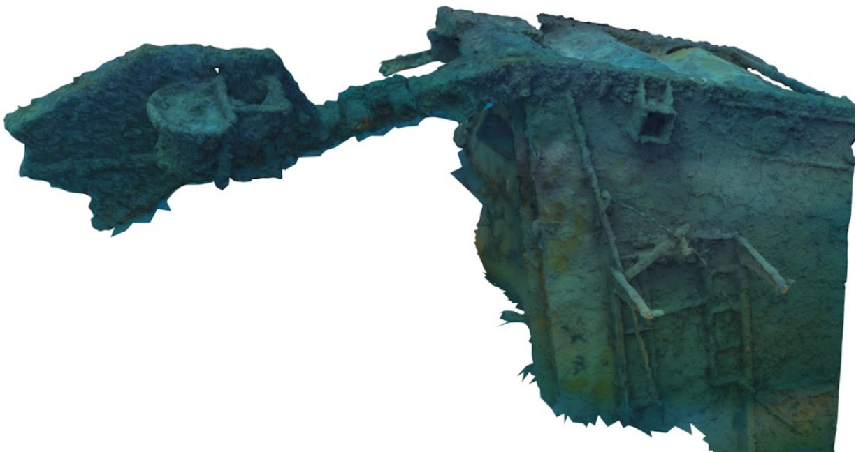
Figure 2: section of the southern side of the wreck represented as simplified mesh textured with normal map and displacement map applied. The model shows high morphological complexity even if the mesh is much simpler and therefore is associated with a smaller file.
