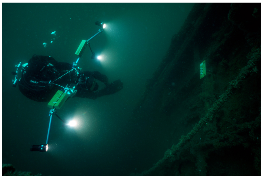
Figure 3.14 - Operator during photogrammetric survey and dimensional reference used to scale the 3D model generated through data analysis.
