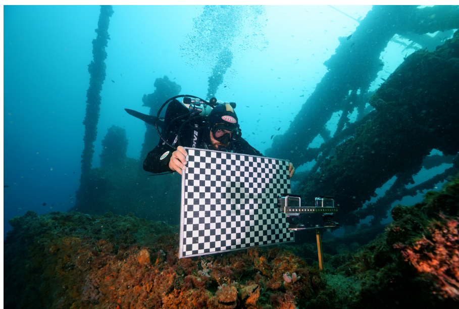
Figure 3.9 - Stereo camera calibration procedure at site.
