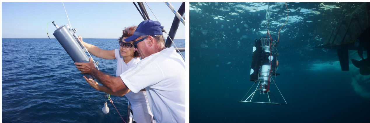
Figure 3.3 - Left: water sampling with Niskin bottle. Right: multi parameter probe during data collection along the water column.
