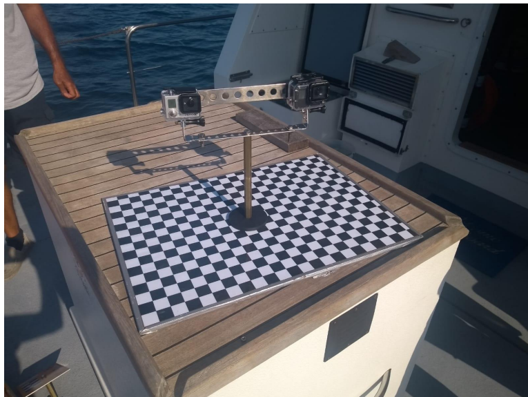
Figure 3.8 - Stereo camera setup and calibration pattern.
