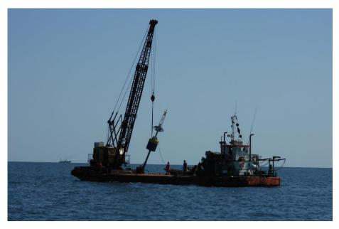
Figure 3.8 - Meteo-oceanographic buoy deployment (May 26, 2021).
