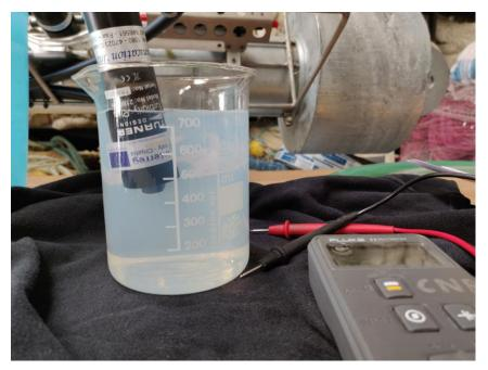
Figure 3.13 - Calibration of turbidity sensor at CNR laboratory.
