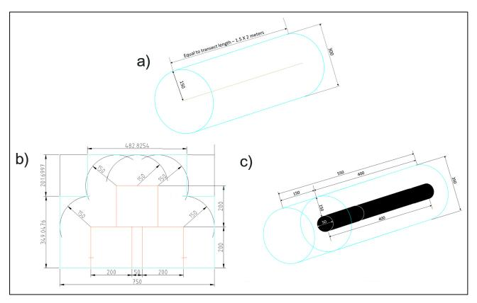
Figure 3.29 - Volume calculation. a: transect; b: pyramid; c: pole. Measures are in cm.
