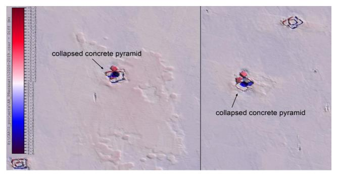
**Figure 2.7** - Difference surface 2020-2018 and the collapse of 2 pyramids. Positive values (in red) highlight concrete blocks that collapsed in 2020, and so sounded in that position only in 2020. Their position in 2018 was in correspondence with negative values (in blue).
