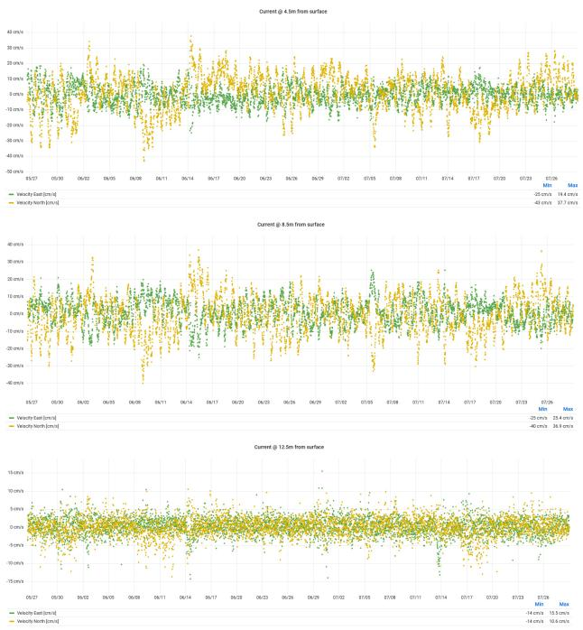
**Figure 4.4** - Time series of eastward and northward currents measured at 4.5 - 8.5 - 12.5 m from the surface. Data were recorded every 20 minutes. Time period: May, 26 2021 - July, 25 2021.
