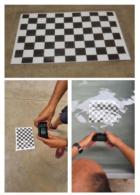
Figure 3.30 - Calibration panel and procedure in air and in water.
