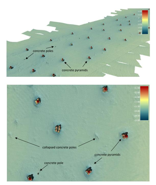
Figure 2.6 - 3D perspective close-up views of the artificial reef and its structures (concrete poles and pyramids).
