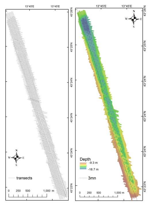
Figure 2.3 - Planning of MBES acoustic survey (left) and hill-shaded bathymetric map (right).
