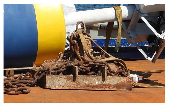
*Figure 3.2* - Mooring system of the buoy composed of a ballast of about 1000 kg and 24 m of iron chain with a diameter of 25 cm.
