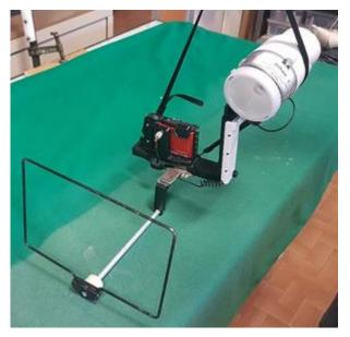
**Figure 3.16** - Nikon COOLPIX W300 digital camera provided with the aluminum frame and underwater speedlight Nikon SB-N10.
