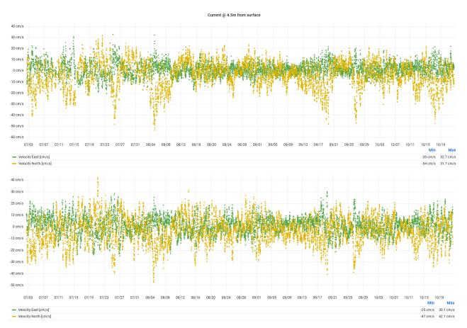
**Figure 4.3** - Time series of eastward and northward currents measured at 4.5 - 8.5 - 12.5 m from the surface. Data were recorded every 20 minutes. Time period: July, 2 2020 - October, 22 2020.
