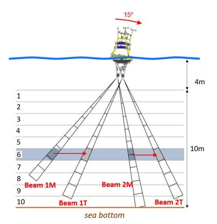
**Figure 3.3** - Vertical arrangement of the cells from the surface to the bottom and example of translation of the measure from field measures (beam 1M and 2M) to true values (Beam 1T and 2T). The translation is automatically calculated by the ADCP through AHRS and its internal magnetometer and accelerometer. Modified from Velasco et al., 2018.
