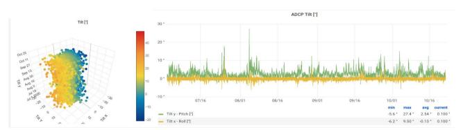
**Figure 3.10** - Compact meteo station (left) and ADCP (right) tilt time series during deployment in 2020. The figure shows the oscillations (pitch and roll) of the buoy caused by the wave motion.
