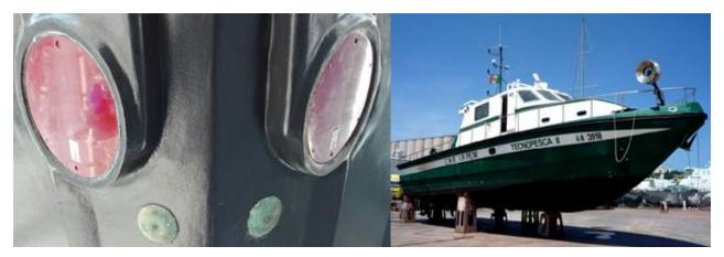
Figure 2.1 - EM2040DC multibeam echosounder (left) hull-mounted on R/V "Tecnopesca I" (right).
