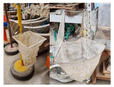
**Figure 3.19** - Photo of the frames used for the scraping sampling: on the left a regular frame 40x40 utilized on the pyramids; on the right the curved frame 30x40 used on the poles.
