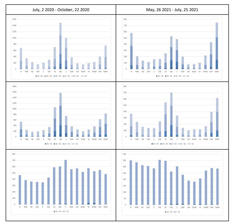
**Figure 4.5** - Occurrences of the water current intensities [cm/s] measured by the ADCP currentometer at 4.5, 8.5 and 12.5m from the surface. The first line indicates the reference period.
