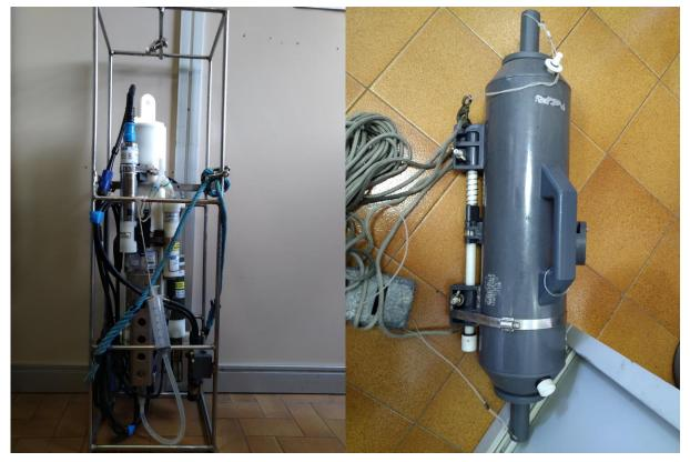
Figure 3.12 - CTD SBE19 plus (left) and Niskin bottle (right).
