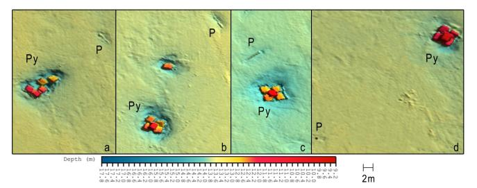
**Figure 2.4** - Structures of the reef of Porto Recanati – Porto Potenza Picena: 2-layer pyramids (Py) and poles (P). Examples of a collapsed pyramid (a) and collapsed poles (a, b and c), a not-intact pyramid (b), two undamaged pyramids (c and d) and a standing pole (d).
