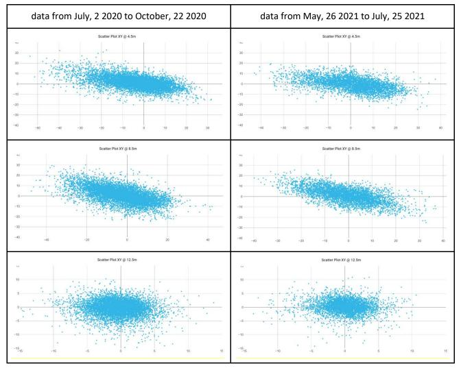
**Figure 4.2** - Currents measured by the ADCP currentometer at 4.5, 8.5 and 12.5 m (top to bottom) from the surface over the time periods July, 2 2020 - October, 22 2020 and May, 26 2021 - July, 25 2021.
