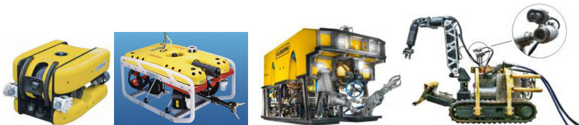
Typologies of ROVs: Observation ROV, Work-Class ROV, Special-use ROV (from left to right) (from https://www.lerus.com.sa/bloa/offshore-operations ).
