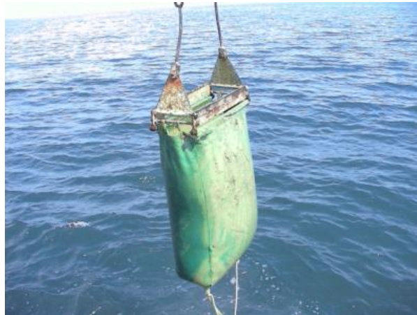
Figure 7: Example of dredge to sample soft-benthic fauna (courtesy of CNR-IRBIM Ancona).
