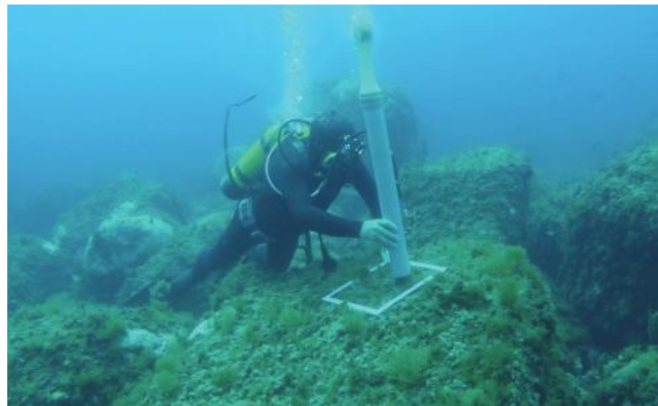
Figure 8: Example of zoobenthic sampling using a suction sampler (from Sciuto et al., 2017).
