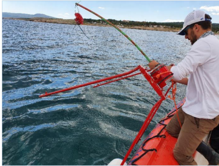
Deployment of the BRUV system in Croatian CSs (Pejdo et al., 2021).
