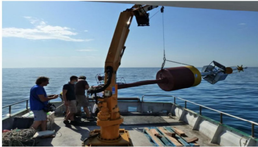
Fixed near-real time oceanographic buoy deployed at Porto Recanati-Porto Potenza Picena (Fabi et al., 2021)
