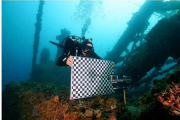
Stereo camera calibration procedure at Paguro wreck and a video processing snapshot with automatic fish detections in overlay.
