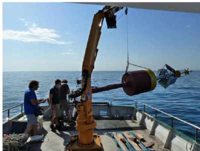
Fixed near-real time oceanographic buoy deployed at Porto Recanati-Porto Potenza Picena (Fabi et al., 2021)
