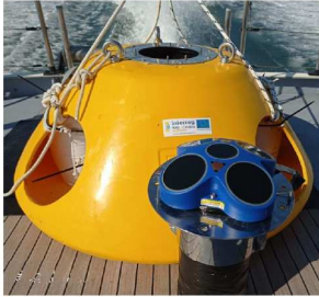
vADCP with the bottom-mount resinex barnacle used at Paguro wreck
