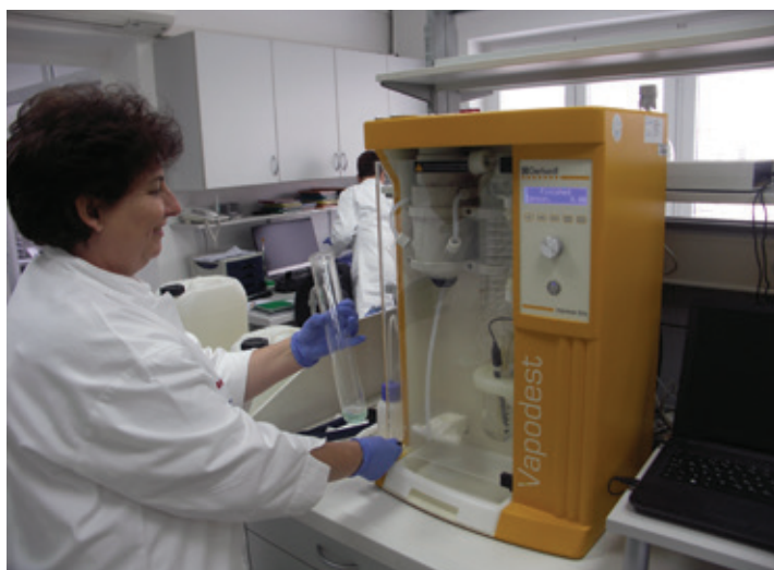
Distillation and titration in the assessment of protein content by Kjeldahl
