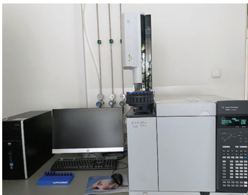
Gas chromatograph with flame ionization detection (GC-FID) for testing the composition of fatty acids
