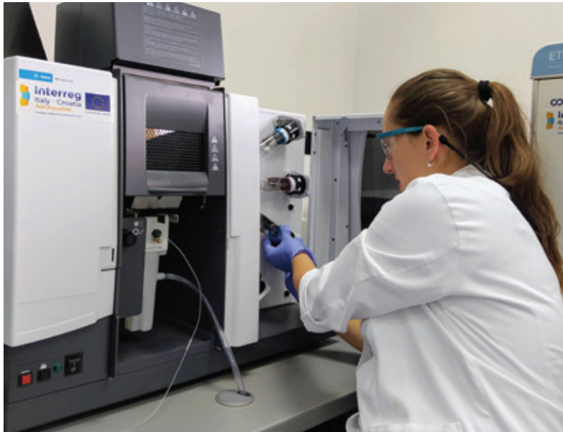
Atomic absorption spectrometry (AAS) for mineral determination
