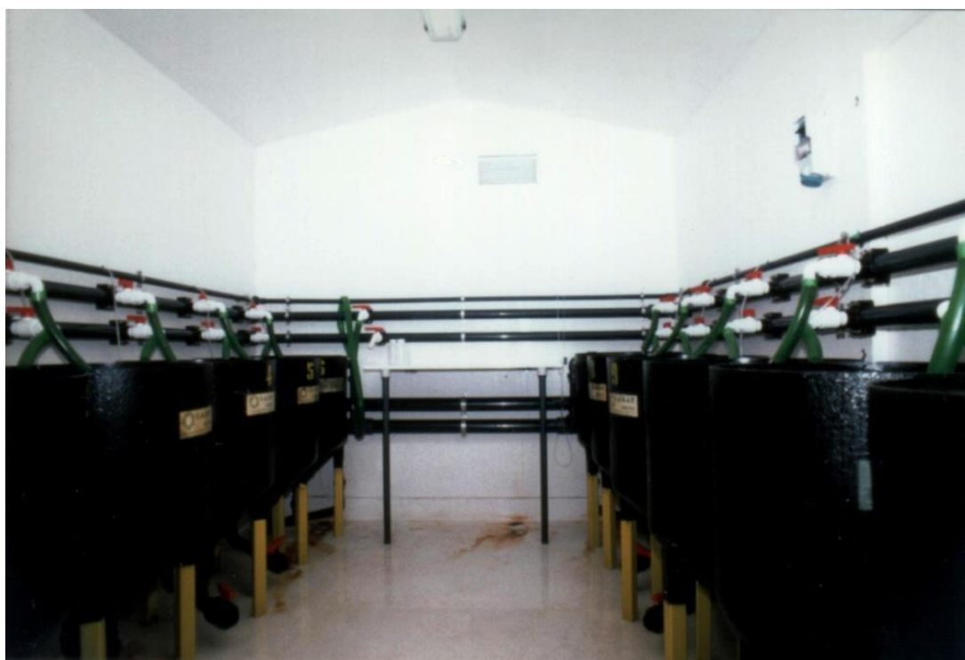
Fig. 8. Experimental tanks being part of an indoor freshwater/sea water recirculating/open system supplied with filtered and UV-treated sea water/fresh water for fish rearing and infection at the University of Udine.
