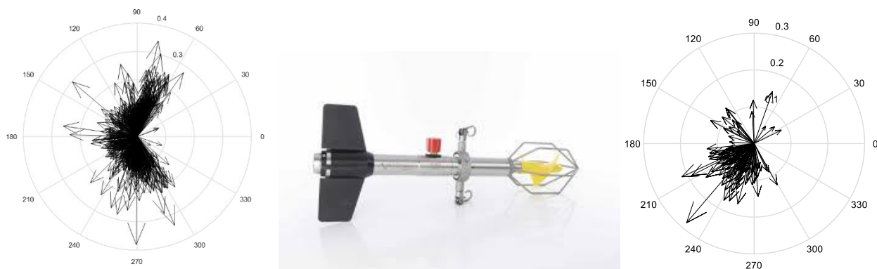
Figure 14. Current velocity [ m s^{-1} ] at the two pilot sites (sx Orada; dx Friskina), recorded by means of current meter, Valeport model 106.
