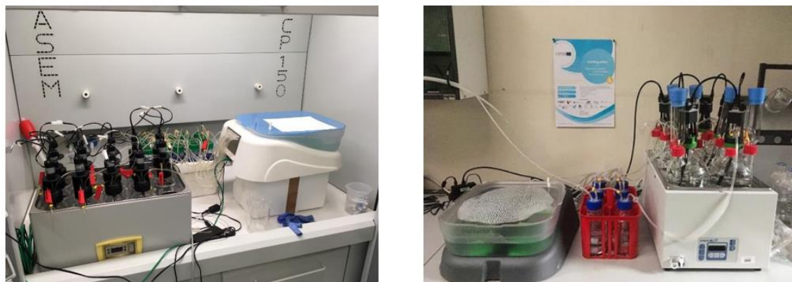
Figure 5. The AMPTS automatic methane potential test system (Lab-scale, on the left) and the BRS bioreactor simulator system (the Pilot-scale system, on the right). The BRS is acquired in the frame of the Adriaquanet Project.
