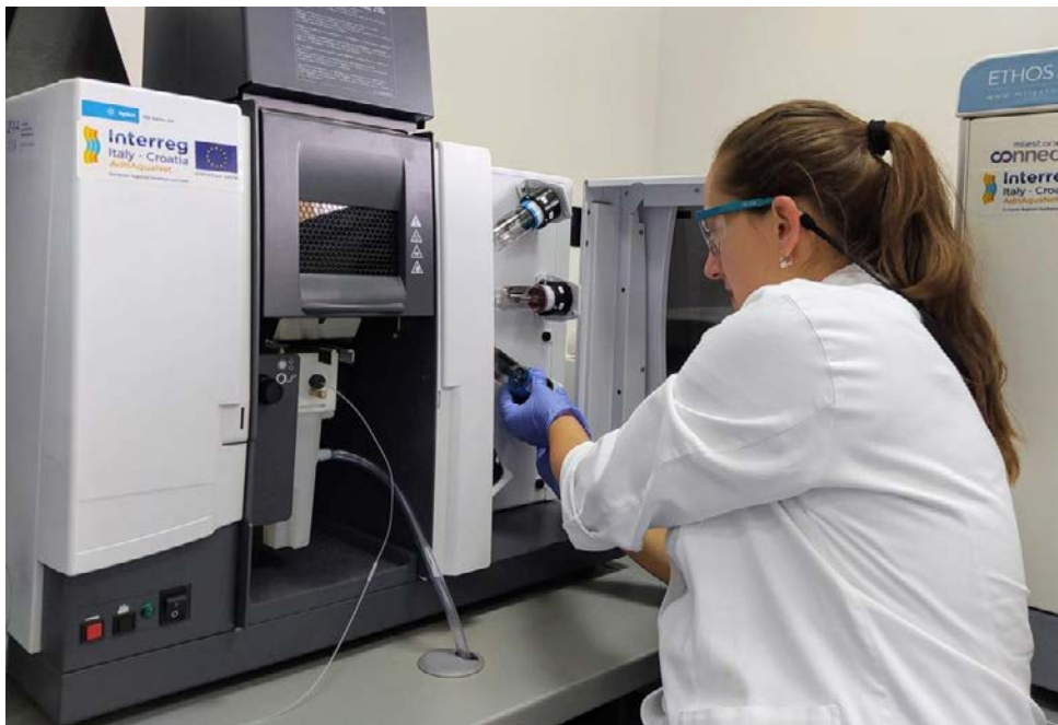
Figure 2 Atomic absorption spectrometry (AAS) for minerals determination.
