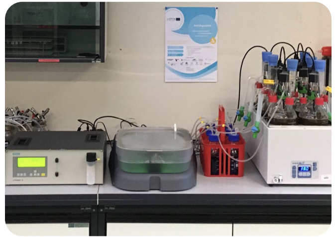
The bioreactor simulator system (BRS, by Bioprocesscontrol) used by LP at Udine University laboratories for pilot-scale tests on anaerobic digestion of fish sludges within WP 3.2.
