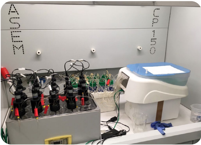
The automatic methane potential test system (AMPTS, by Bioprocesscontrol) used by LP at Udine University laboratories for lab-scale biochemical methane potential (BMP) determination within WP 3.2.
