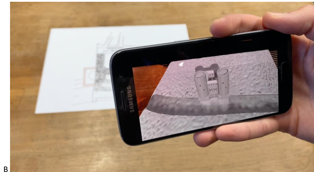
Figure 1: Figure a shows the 3D model of the city gate of Altino. The modeling of the city gate was carried out in Blender 2.83, an open source software. The geometry of the elevation has been represented applying the principle of Level Of Details. To improve the interaction between the final user and the 2D - 3D information, an Augmented Reality application (Figure b) was realized with Unity 2019.4. This app allows to frame with a device the edited planimetry and to extrude the virtual model.
