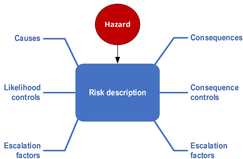
Figure 4 The basic BowTie diagram
