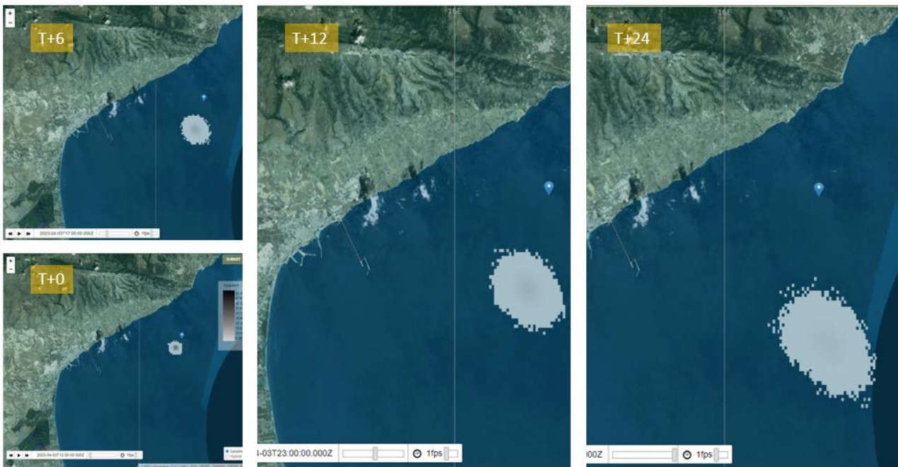
Im. 37: The Witoil platform developed in the FIRESPELL project. 1000t oil spill simulation using current forecasting models (IFS – ECMWF and Med Sea – CMEMS). The model determines the spread, the density (tons/km 2 ), and the movement of the oil.
