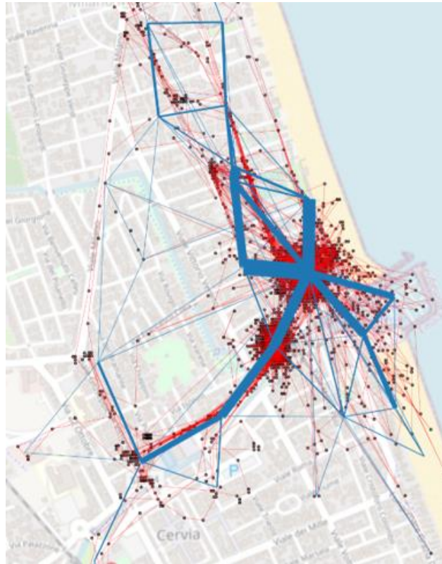
Figure 11. Example of the “cloud of points” generated from the GPS system when it stopped in a place. In blue it is possible to see how a dedicated algorithm allowed to transform and clean these data into more realistic one.
