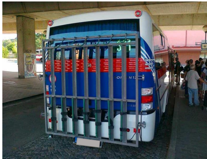
Figure 39 - Backside racks in Czech Republic with raised bicycles (source: Cerny and Daggars, 2016)
