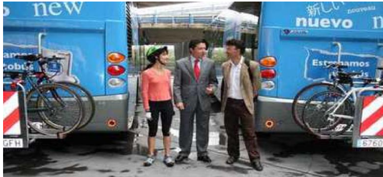
Figure 40 - Rear racks in Spain with bicycles on the racks (source: Cerny and Daggars, 2016)
