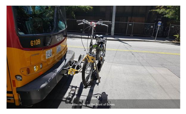
Figure 38 - Bike racks on the front of city buses (<a href="https://cycle-works.com/products/bus-racks/">https://cycle-works.com/products/bus-racks/</a>)
