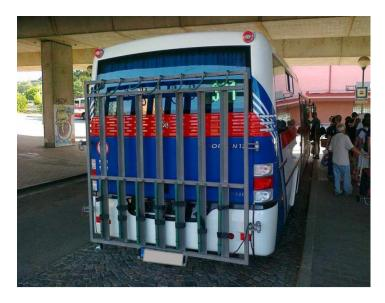
Figure 39 - Backside racks in Czech Republic with raised bicycles (source: Cerny and Daggers, 2016)
