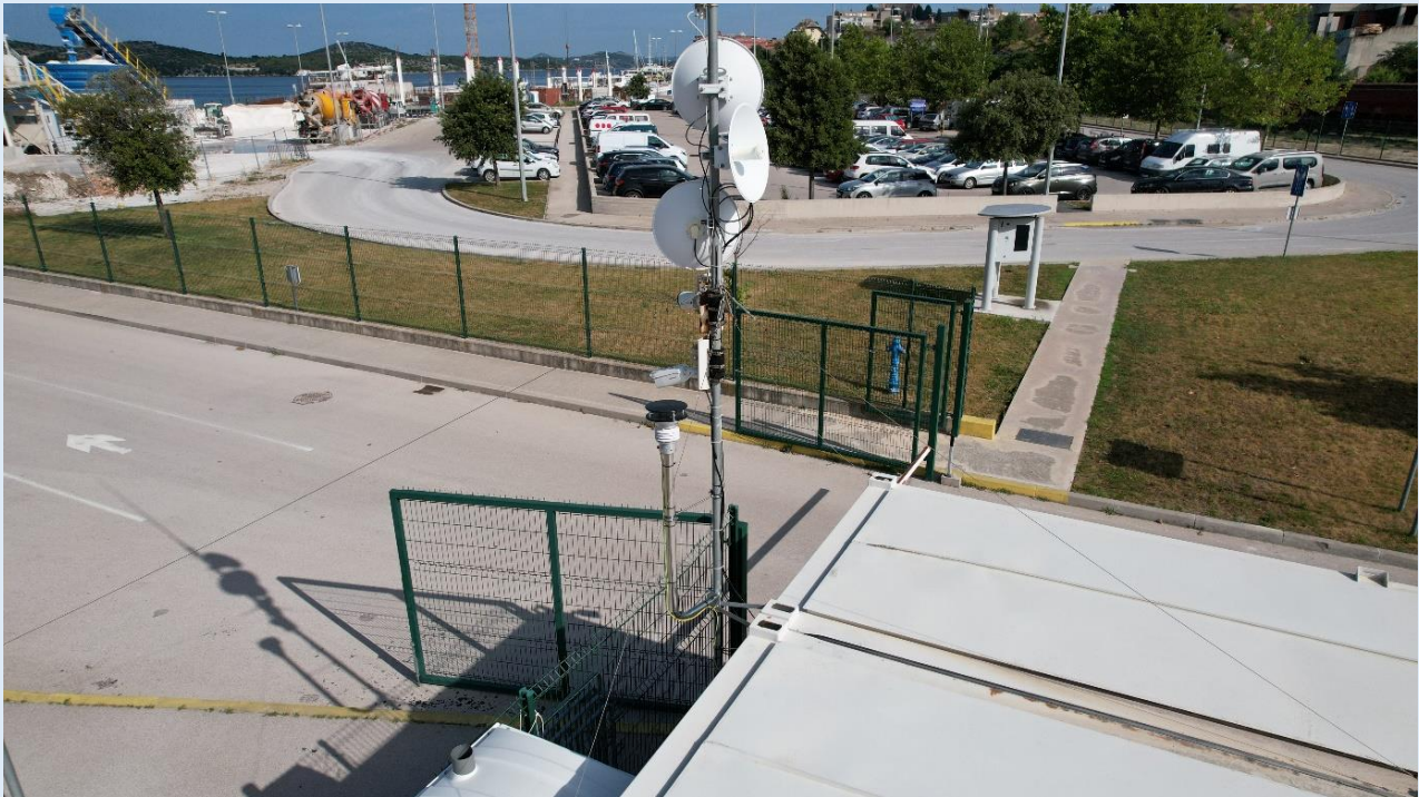
Figure 15. Land sensors for receiving information from buoys 2 (photo made by air drone)
