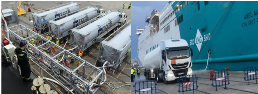
Figure 66: Bunkering in truck-to-ship mode (Source: Snam s.p.a.)
