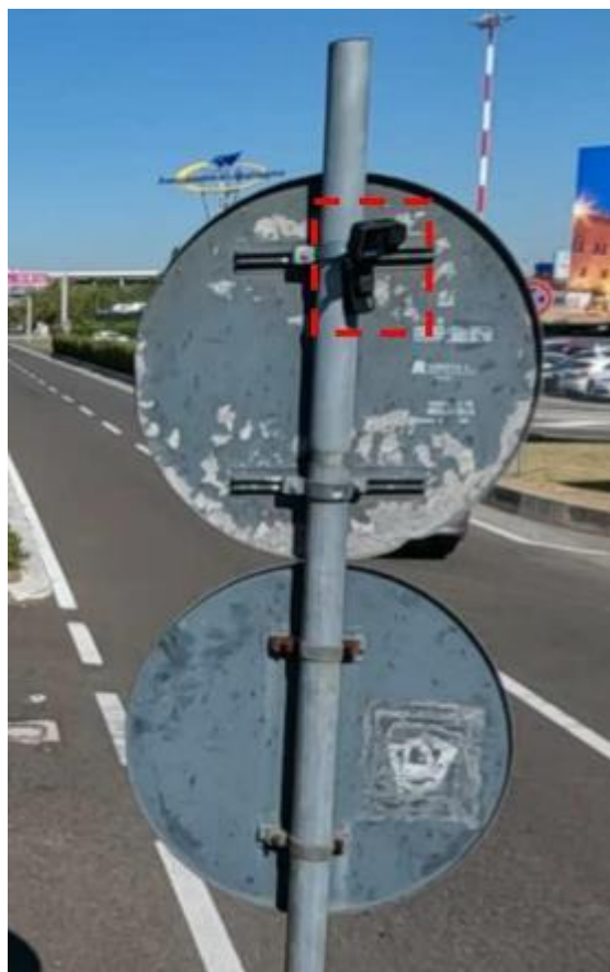
Figure 10. Picture showing the GoPro Hero 10 camera attached to a pole with a magnetic support.
