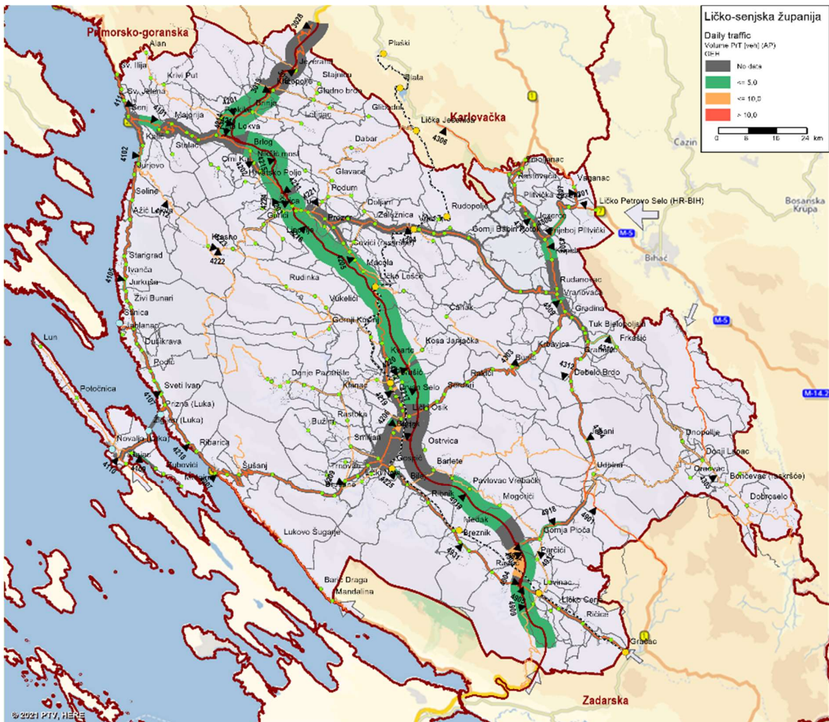
Picture 23. The validation of traffic load according to the statistical GEH values analysis, off-season
