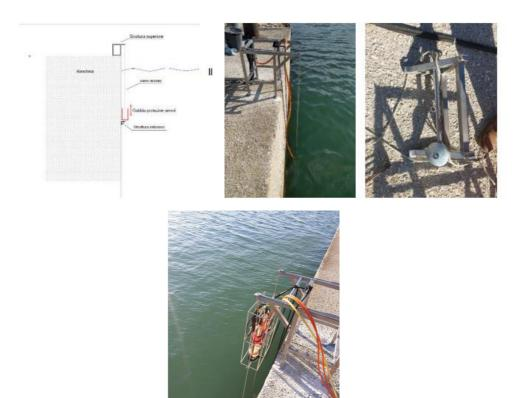
The power system, collecting and sending data was installed in the immediate vicinity of the probe. It is composed of a support structure built in 316 stainless steel on which they are located housing all the components necessary for the stowage of the batteries and subsystems related to the data collection and transmission system.
