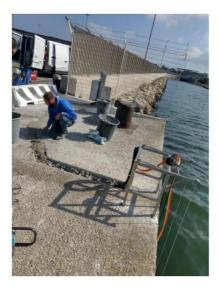
The system is currently configured to collect data relating to pressure, conductivity, temperature, dissolved oxygen, turbidity and chlorophyll at frequencies of 2Hz for 1 minute every 30 minutes.
