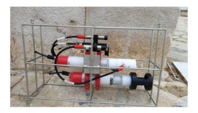
The power system, collecting and sending data was installed in the immediate vicinity of the probe. It is composed of a support structure built in 316 stainless steel on which they are located housing
