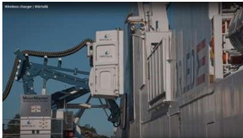
Figure 11: View of the WI-FI ferry charger of the Finnish manufacturer Wärtsilä Source: Wartsila officel website
