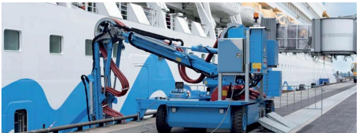
Figure 6. Quick and easy connection to the ship via the cable management system
