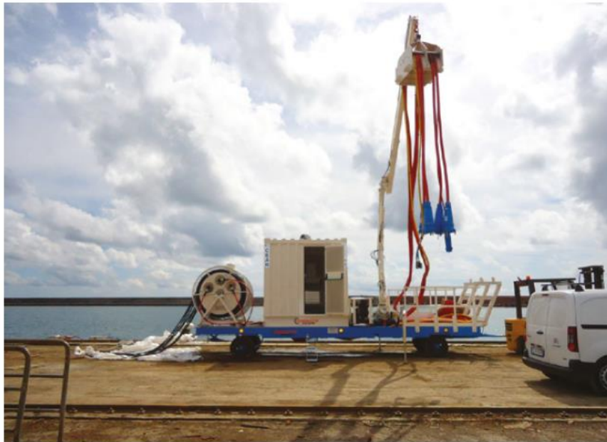
Figure 7 - Mobile structure for powering ships (Source: Port System Authority of the Western Ligurian Sea)
