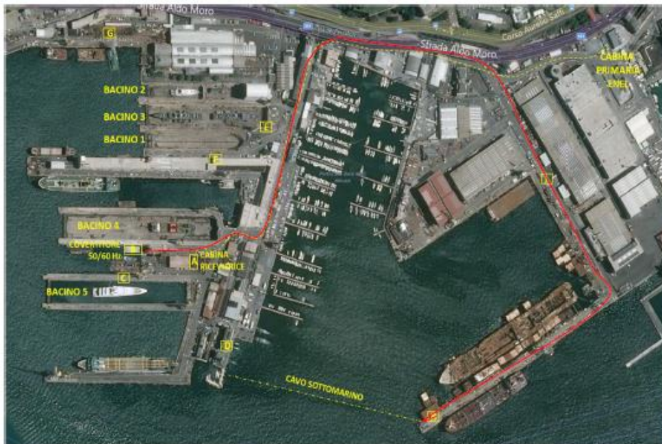
Figure 8 - Submarine cable vs the construction of a conduit in the dry docks (the red line) (Source: Port System Authority of the Western Ligurian Sea)
