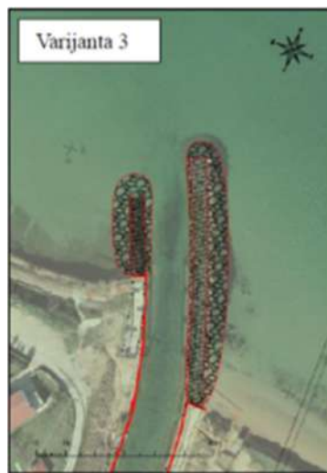
Figure 71 The analysed variant solution of Miljašić Jaruga river mouth (variant 3 - both groynes as combination of vertical wall type and sloped rock armour)
