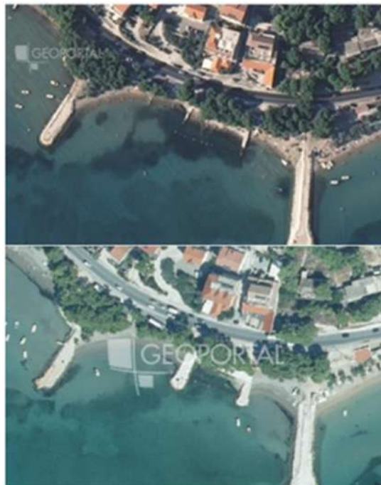
Figure 92. Example of changes in the meadows area and structure between 2014 and 2017 which were estimated as being caused by dikes construction on the shoreline.
