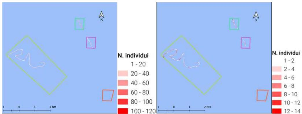
Figure 52. Map of the target density detected within the December campaign – darker colour is associated to a higher target density within the 200m segment. Left: entire dataset; right: TS > -65db.
