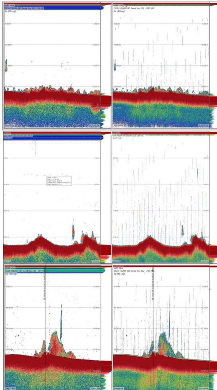
Figure 51. Examples of echograms detected during the campaigns, at the 38 kHz frequency. Top panel: December 2021, area 3, concentration of targets close to the bottom (possible demersal organisms); central panel: January 2022, area 1, possible demersal organisms close to the bottom; bottom panel: March 2022: concentration of targets above a Tegnùà.
