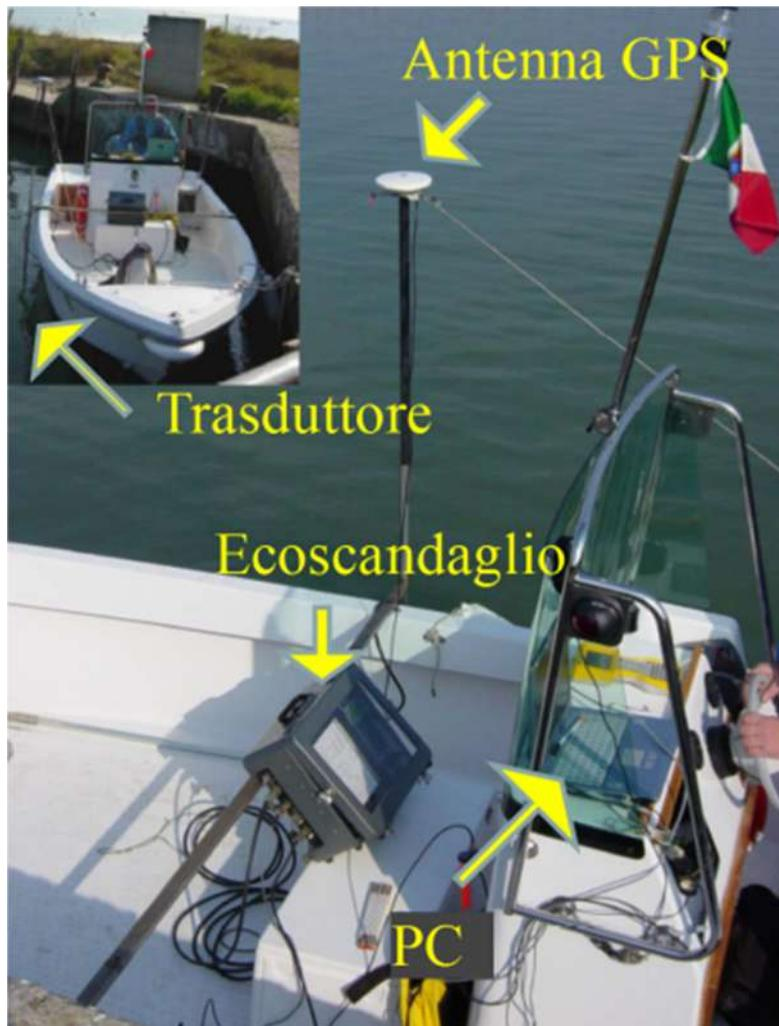
Figure 14. Boat used for the survey, equipped with the necessary instruments.
