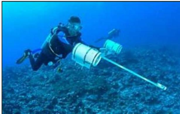
Figure 58. Stereo BRUV used with the help of a diver.
