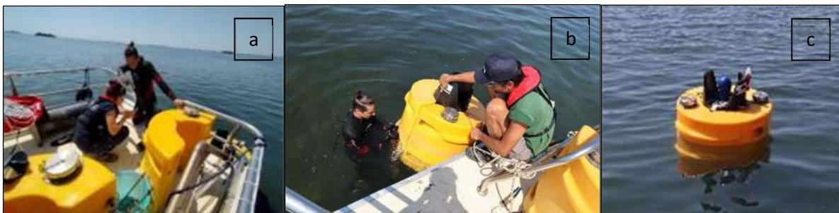
Figure 3. Some pictures taken during the installation: a) configuration of the instruments; b) anchoring; c) the site at the end of installation.
