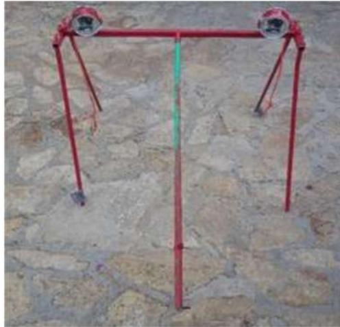
Figure 59. Stereo BRUV system used in the research.
